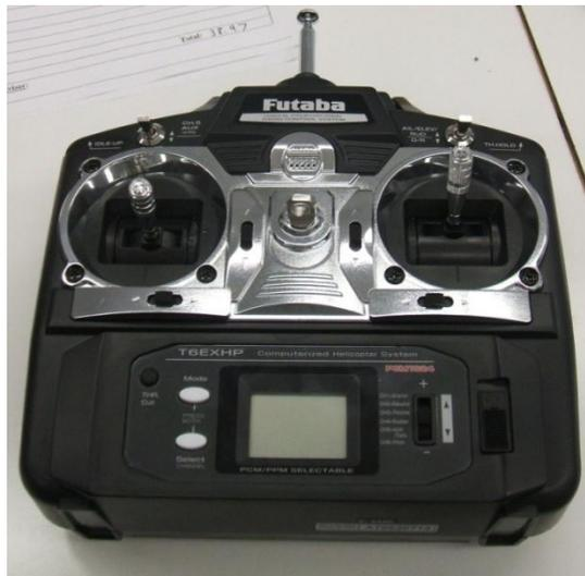
Figure 3.7: Futaba 6EXH Computer Transmitter 72MHz
