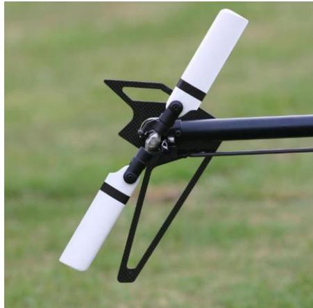
**Figure 2.4: R/C helicopter tail rotor [5]**
