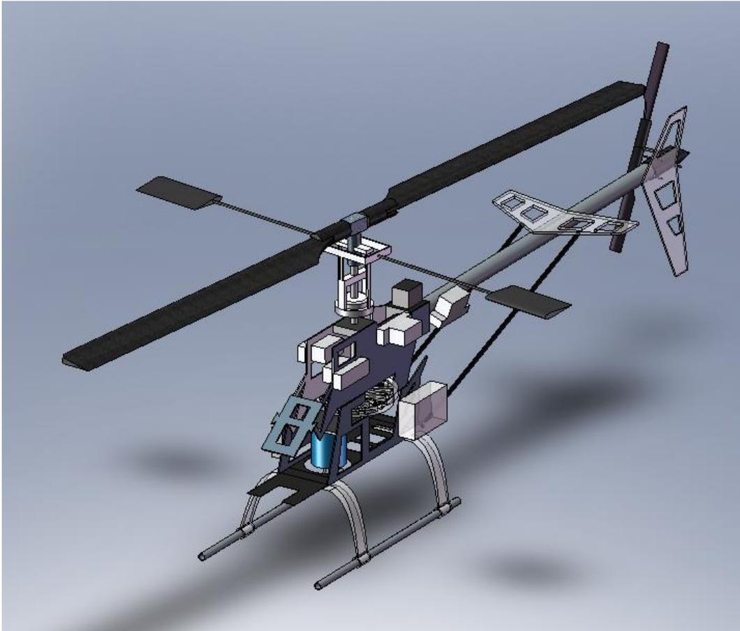
**Figure 5.2: SolidWorks model of helicopter**
