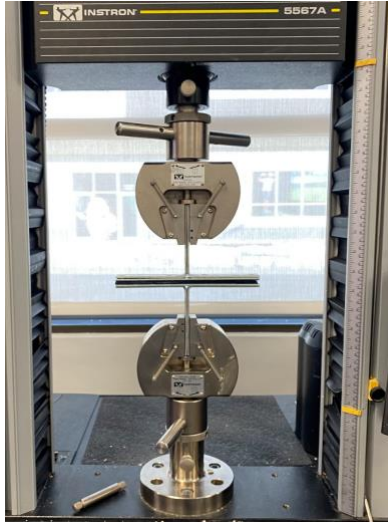
Figure 13: Set up procedure for tension test
