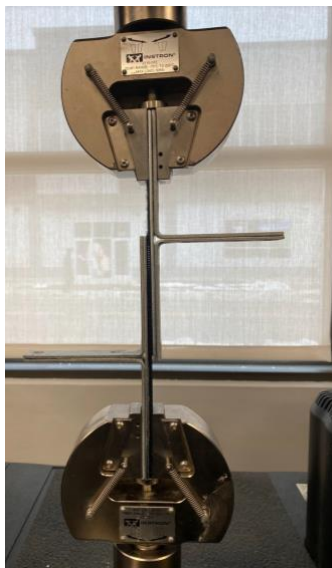
Figure 14: Set up procedure for shear test
