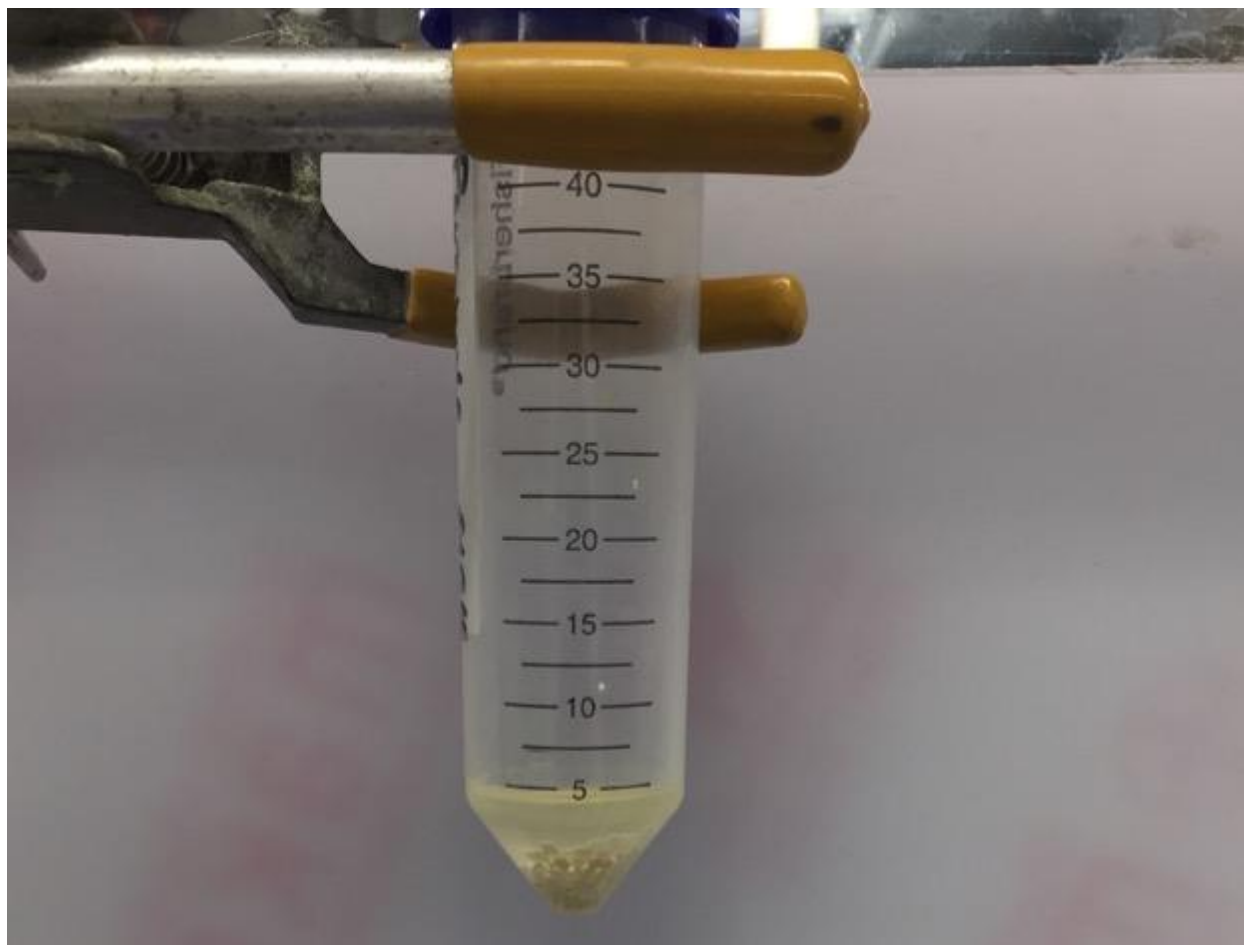
Figure 33: Eggshells, Peroxide, 24 hours, 1.0 g catalyst, EtOH, Stirred, 27 hours
