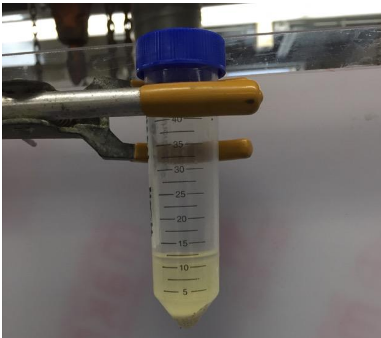
Figure 32: Eggshells, Bleach, 24 hours, 1.0 g catalyst, MeOH, Stirred, 27 hours.
