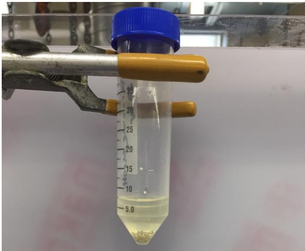
Figure 35: Eggshells, Peroxide, 24 hours, 1.0 g catalyst, MeOH, Stirred, 27 hours
