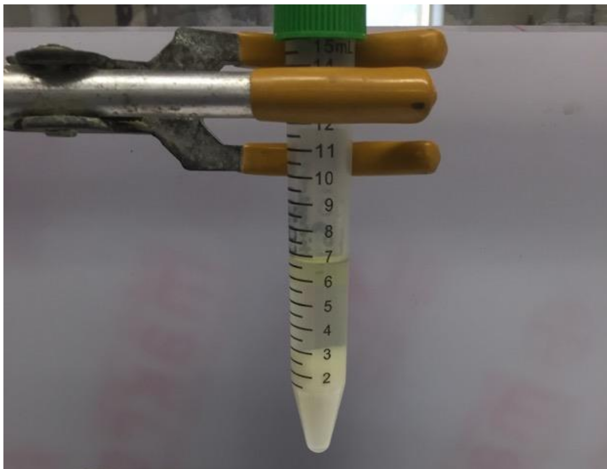
Figure 41: Eggshells, 900°C, 3 hours, 1.0 g catalyst, MeOH, Stirred, 24 hours
