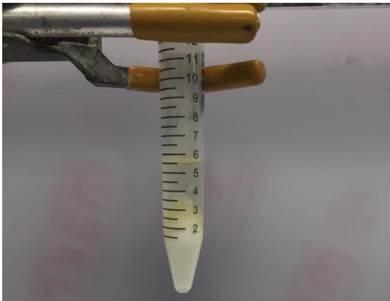
Figure 40: Eggshells, 400°C, 6 hours, 900°C, 6 hours, 1.0 g catalyst, MeOH, Stirred, 22 hours.
