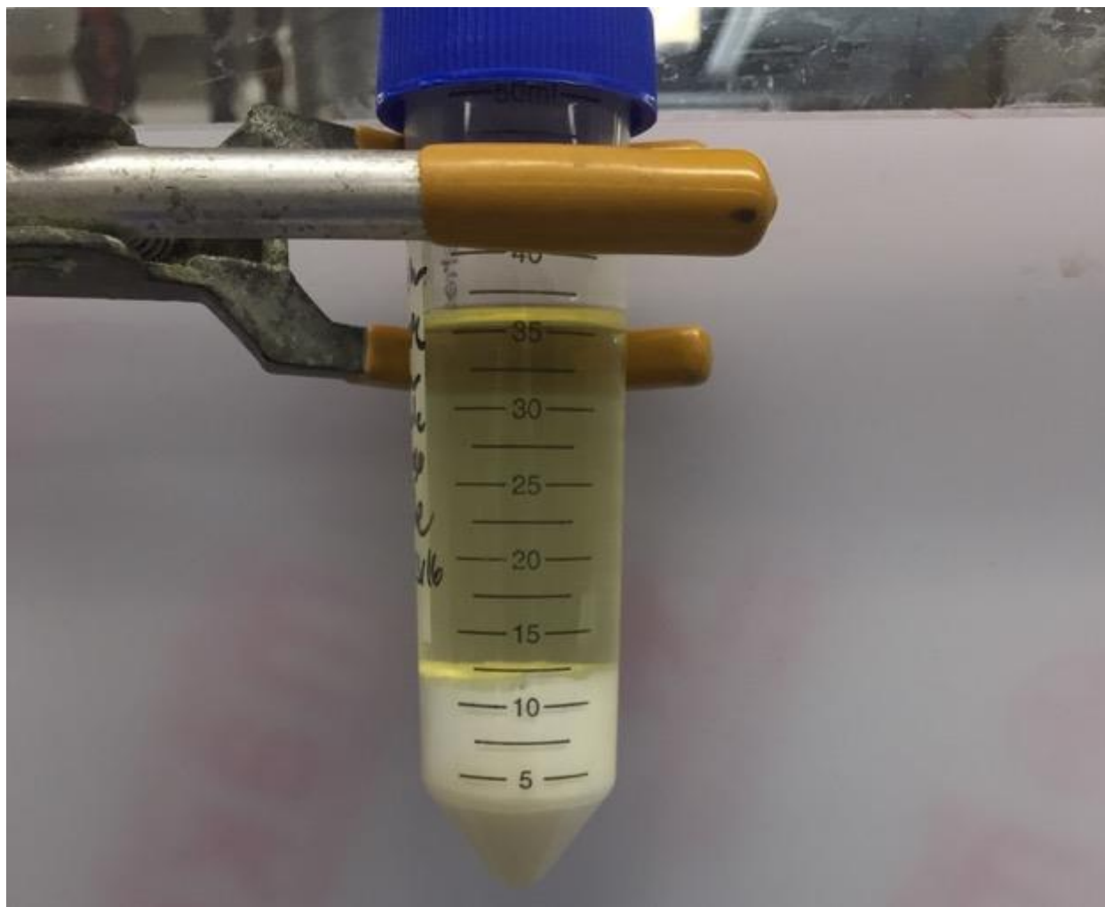
Figure 36: Eggshells, 900°C, 3 hours, 1.0 g catalyst, EtOH, Stirred, 24 hours.
