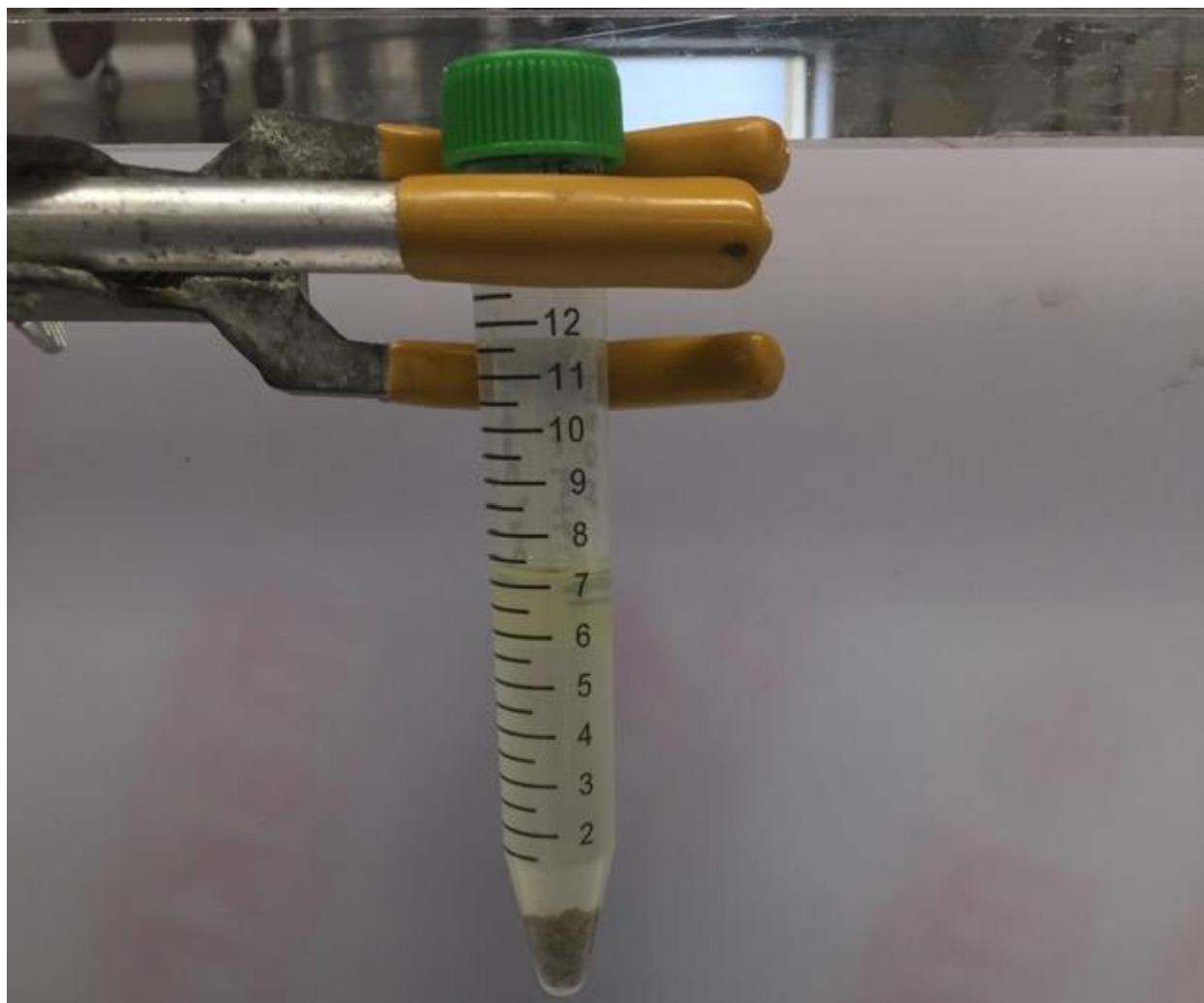
Figure 42: Eggshells, 400°C, 6 hours, 1.0 g catalyst, MeOH, Oscillating Water bath (35°C), 24 hour.
