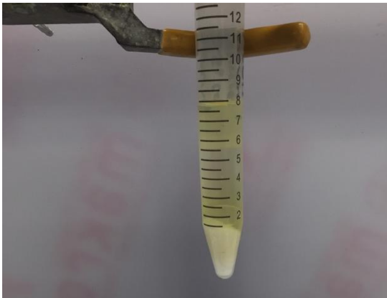
Figure 38: Eggshells, 400°C, 6 hours, 900°C, 6 hours, 0.5 g catalyst, MeOH, Stirred, 22 hours.
