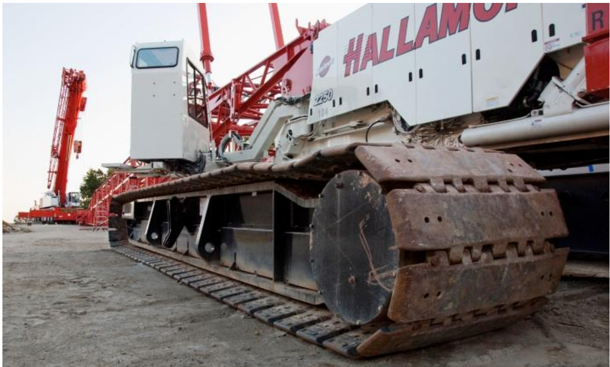
Figure 28: Shows the Manitowoc 2250 Crane which requires a 26 foot width access road
