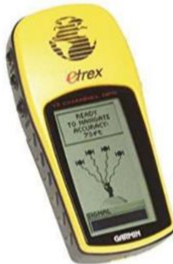
Figure 3.3. The Garmin eTrex H GPS, used to note elevation and coordinates for all photopoints (Conroy, 2018).
