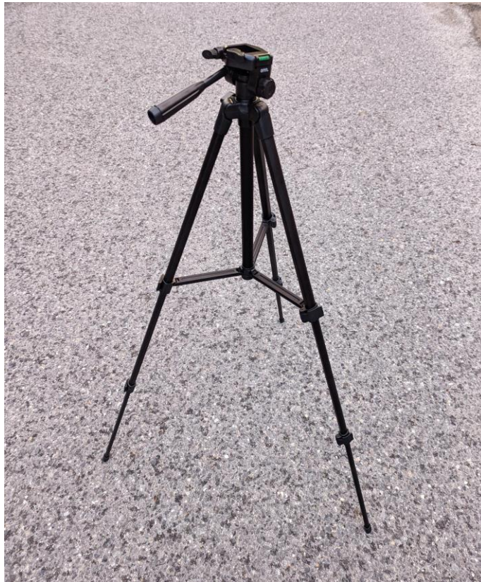
Figure A.3. The Onn 52" Lightweight Tripod, used to stabilize the Lumix and hold it at a controlled height and angle. (Taken by Vinh Tran)
