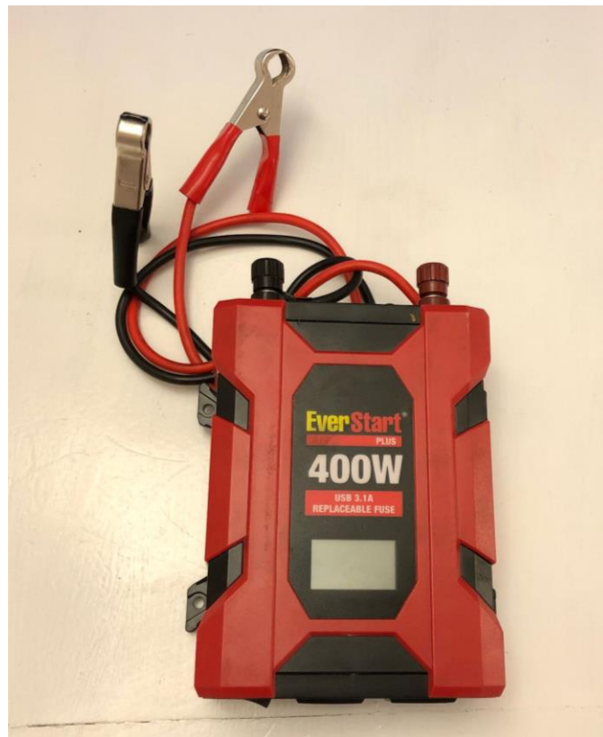
Figure A.12. EverStart 400 Watts Vehicle Power Inverter Converter 12V DC to 110V AC. (Taken by Ryan)
