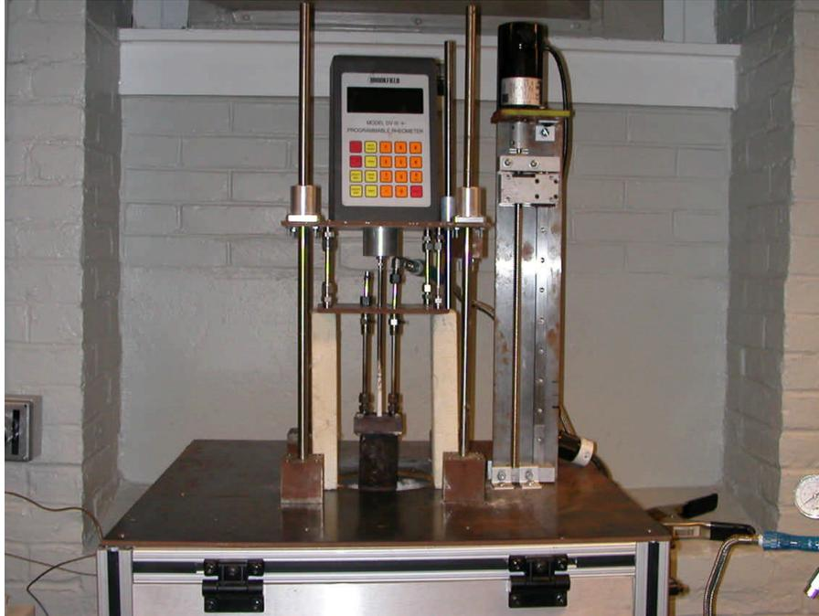
**Figure 21 - Dendrite Coherency Apparatus.**
