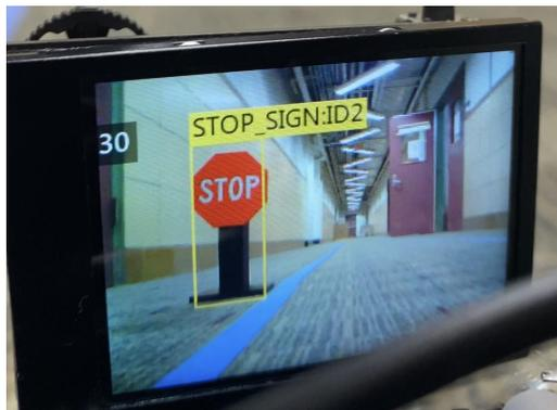
Figure 9.6: HuskyLens Correctly Detecting Road Sign
