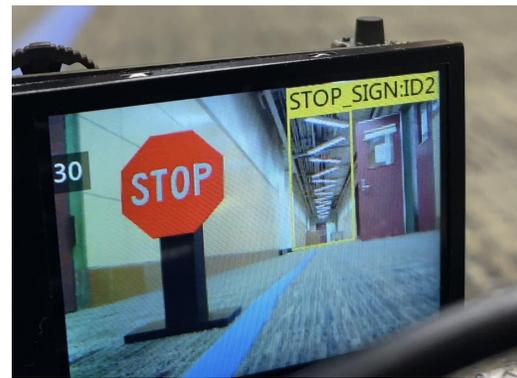
Figure 9.7: HuskyLens Falsely Detecting Ceiling Lights as Road Sign
