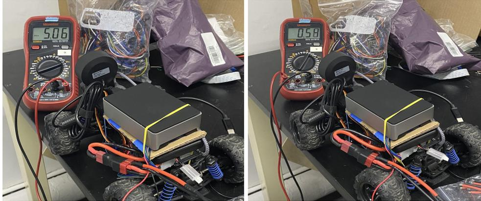
Figure 7.6: LiPo Power Circuit Multimeter Testing
