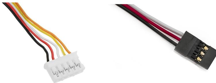
Figure 11.3: 5-wire Servo vs 3-wire Servo
