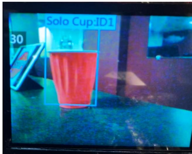
Figure 9.2: HuskyLens Object Recognition Testing
