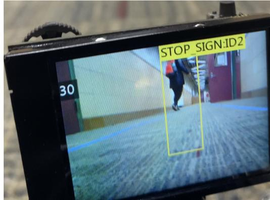
Figure 9.8: HuskyLens Falsely Detecting Red Backpack as Road Sign
