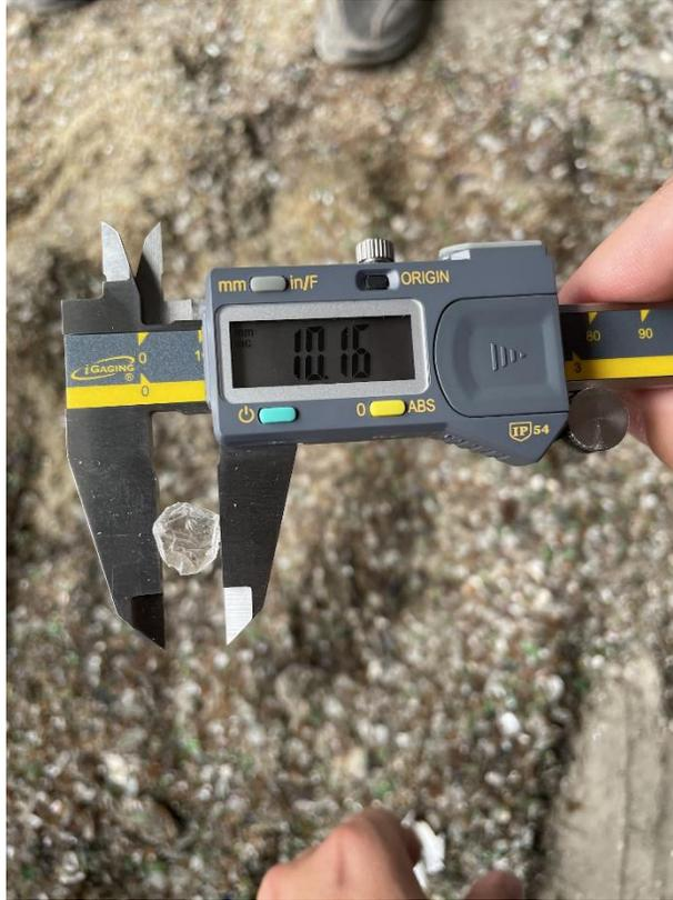
Figure 6: A piece of pulverized glass at Bloques Caribe Inc., measured to be 10.16 mm.
