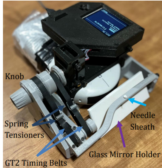
Figure 1. Previous MQP device prototype for PCNL US-guided needle insertion tool [13].
