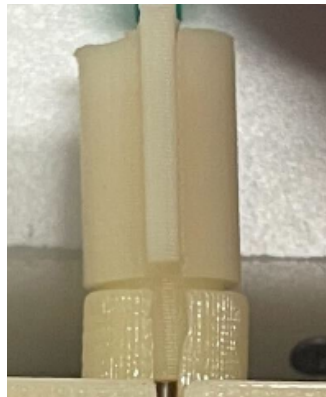
Figure 19. A close-up depicting the slight lift and tilt of the needle lock during testing.
