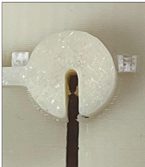
Figure 17. A close-up of the printing error found in the needle relief slot.
