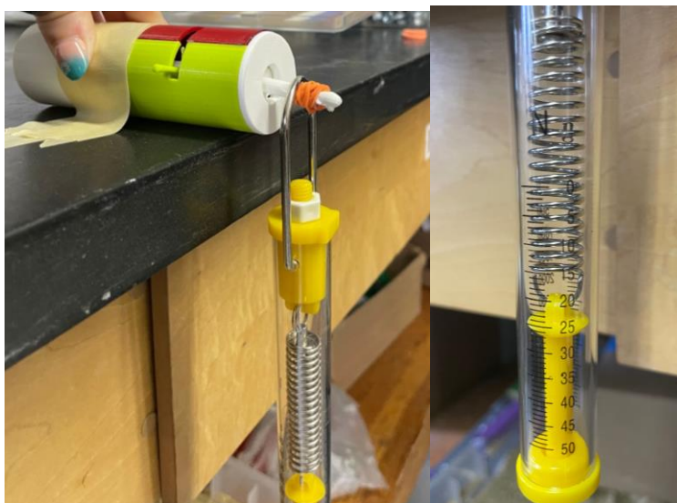
Figure 32. Hook deformation at 25 Newtons.
