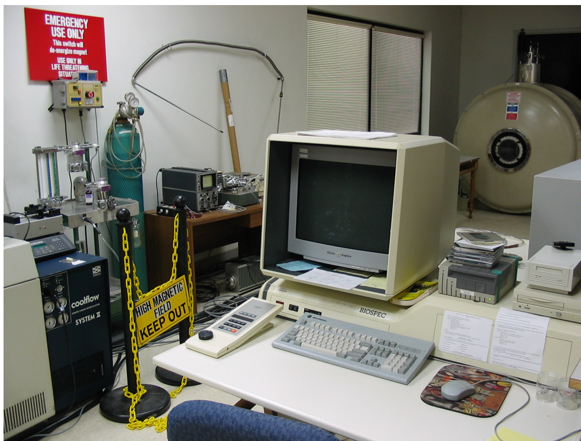
Figure 3-5. Bruker Biospin 2.0T/45cm imaging spectrometer equipped with \pm 20 G/cm self-shielded gradients. Current software: Paravision 2.1.1.
