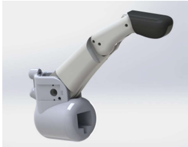
Figure 16: CAD Model of IRIS Finger Design (Casley, S. et al., 2014).
