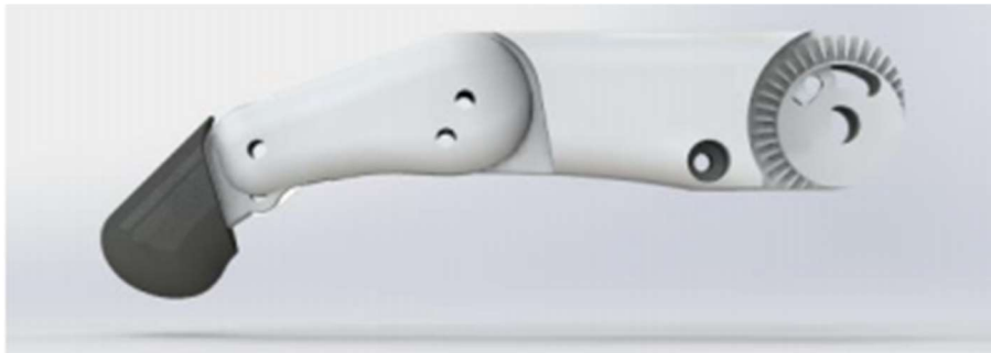
Figure 21: CAD Model for Redesigned Gear-Driven Finger (Edwards, R. et al., 2015).
