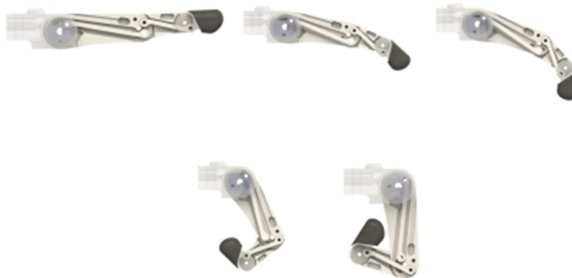
Figure 17: Full Range of Motion of IRIS Finger (Casley, S. et al., 2014).
