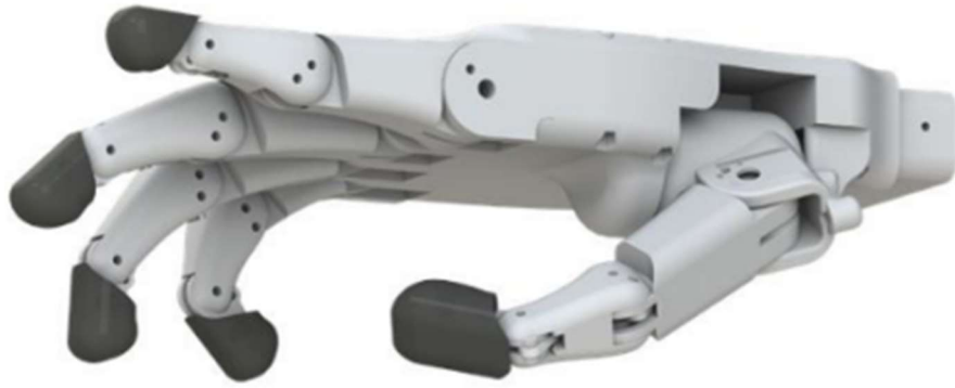
Figure 18: CAD Rendering of IRIS Hand (Casley, S. et al., 2014).
