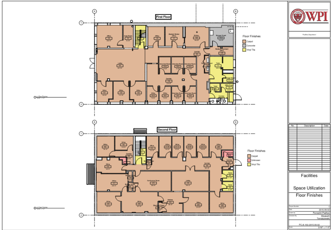
Figure 27: Drawing sheet indicating Floor Finishes
