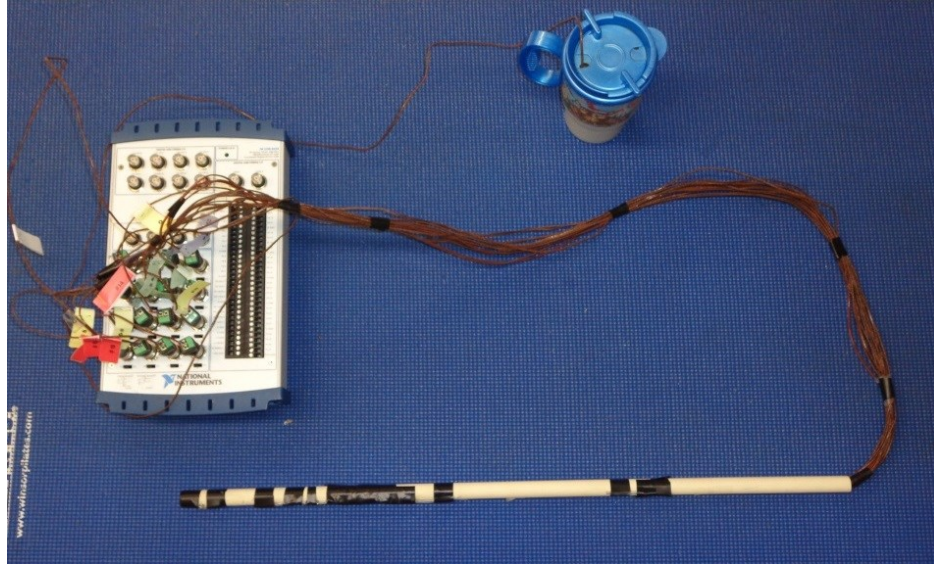
Figure 6.11 Thermocouple tree, CJC and DAQ
