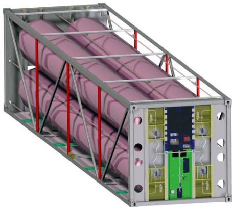
Figure 32 - 5,000psi hydrogen storage tanks 58
