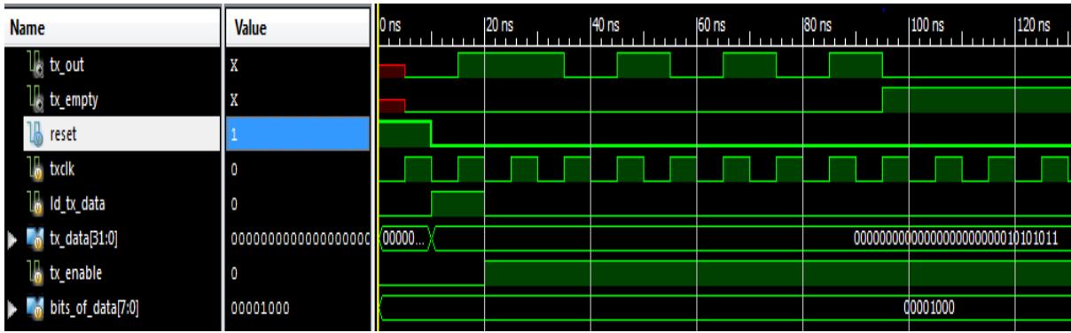
Figure 4.13 Results of TX in simulation (Top to Bottom: Data Out, Transmit Empty (not part of functionality), Reset, Serial Clock (not part of functionality), Load Transmit Data, Data to be transmitted, Transmit Enable, Number of bits of Data)
