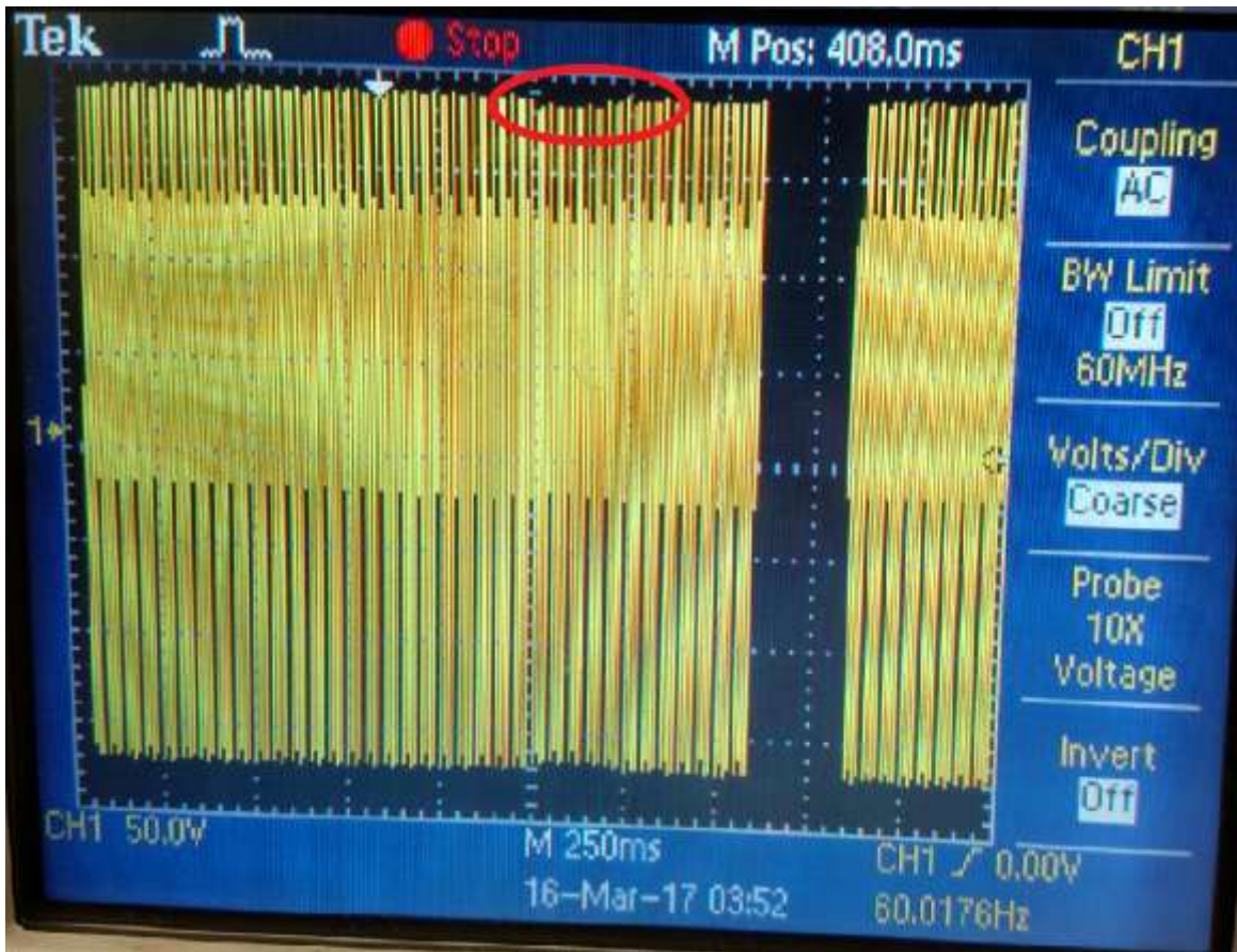
Figure 47. On-Grid Voltage Sag Caused by Motor Operation
