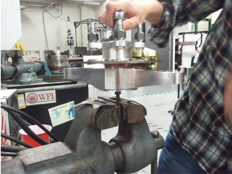
**Figure 44: Hub Assembly Fixture**
