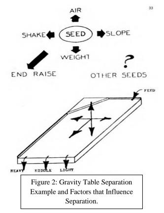
figure 2 (Thomas, 1980). Stratification occurs in a stratifying area where vibration and the light flow of air combine to form layers out of the material from top to bottom following the pattern of low to high specific gravity, respectively. The vibration of the stratification area's surface pushes the heavier layers due to them contacting the surface while the lighter layers float to an exit area for collection.
