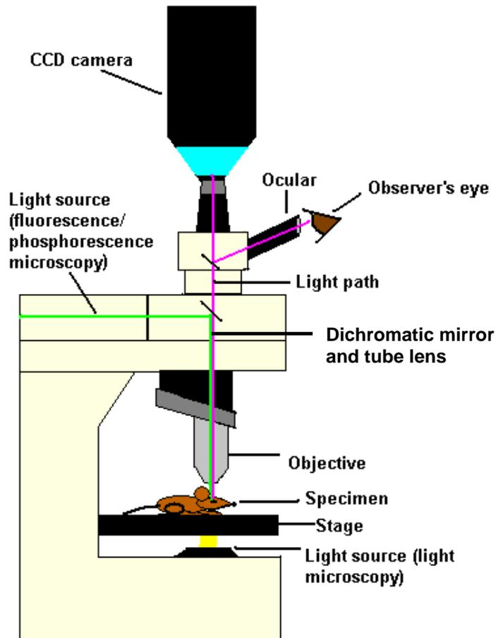
**Figure 2.3-Optical train of a microscope. The specimen is illuminated by one of the light sources, and the image of the specimen travels along the optical train to the camera and/or the observer's eye.**
