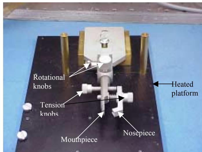
**Figure 3.3—Stereotaxic head holder. Mouse rests on a heated platform, designed to maintain body heat while animal is under anesthesia. The mouthpiece is inserted into the animal's mouth, and the nosepiece is tightened onto the nose with the tension knobs. The rotational knobs are loosened to allow proper positioning of the head so the eye may be viewed, and tightened to prevent movement once the proper position is achieved.**
