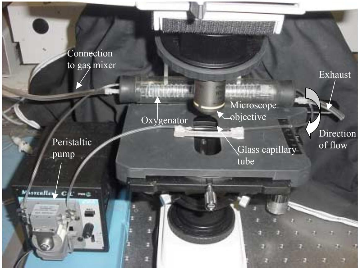
**Figure 3.1—*In vitro* system.** The system consists of an oxygenator connected to a gas mixer, a peristaltic pump used for circulating probe solution inside the system, and a square glass capillary tube situated under the microscope objective used for measuring the  $PO_2$  of the solution. The parts are connected with Tygon® microbore tubing, which may be disconnected at various junctions and injected with solution using a 22-gauge needle and syringe.
