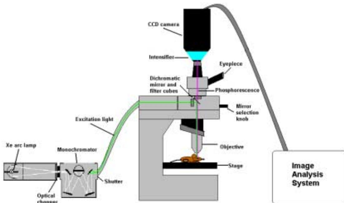
**Figure 2.4-The phosphorescence lifetime imaging system. White light is emitted by the xenon arc lamp and sinusoidally modulated by the optical chopper. The monochromator selects a particular wavelength of light, which is directed to the eye by a dichromatic mirror. Phosphorescence is produced by probe in the eye, and travels to the CCD camera.**
