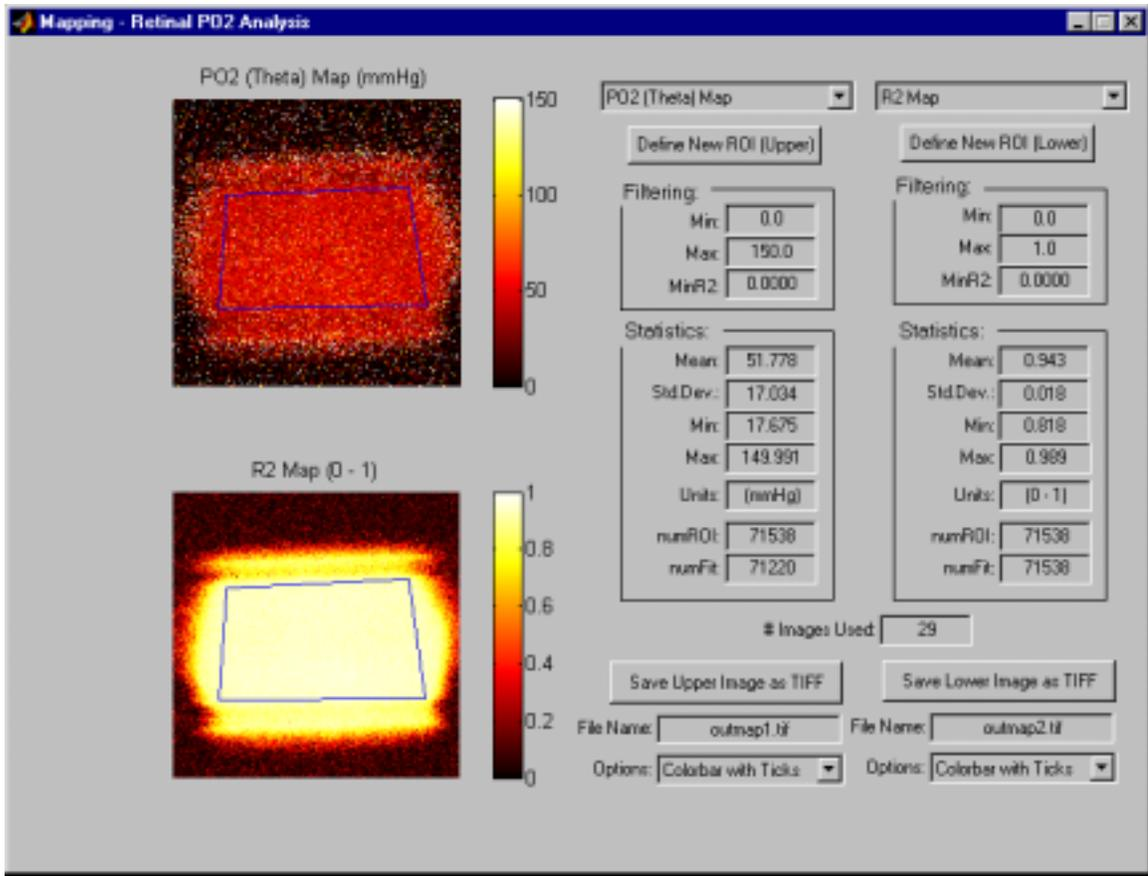
**Figure B.4—“Calculate Maps” screen. A number of different maps may be created using the pull-down menus at the top. Filtering parameters may be input to reduce extraneous pixels in the images. Statistics are output in the right center of the screen.**
