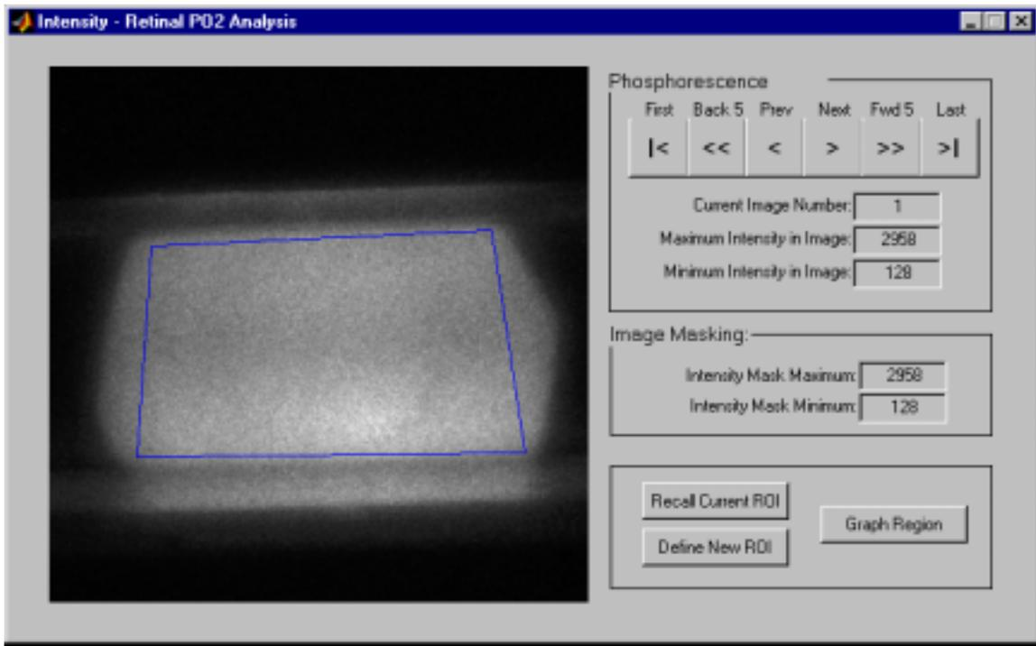
**Figure B.2—“Show Intensity Images” screen. Individual intensity images may be viewed using the buttons at the top of the screen. An ROI may be selected by pressing one of the buttons at the bottom, and using the mouse to define a region on the image—the ROI selected in this image appears in blue. A graph of intensity versus phase delay for the ROI may be created by pressing the “Graph Region” button.**
