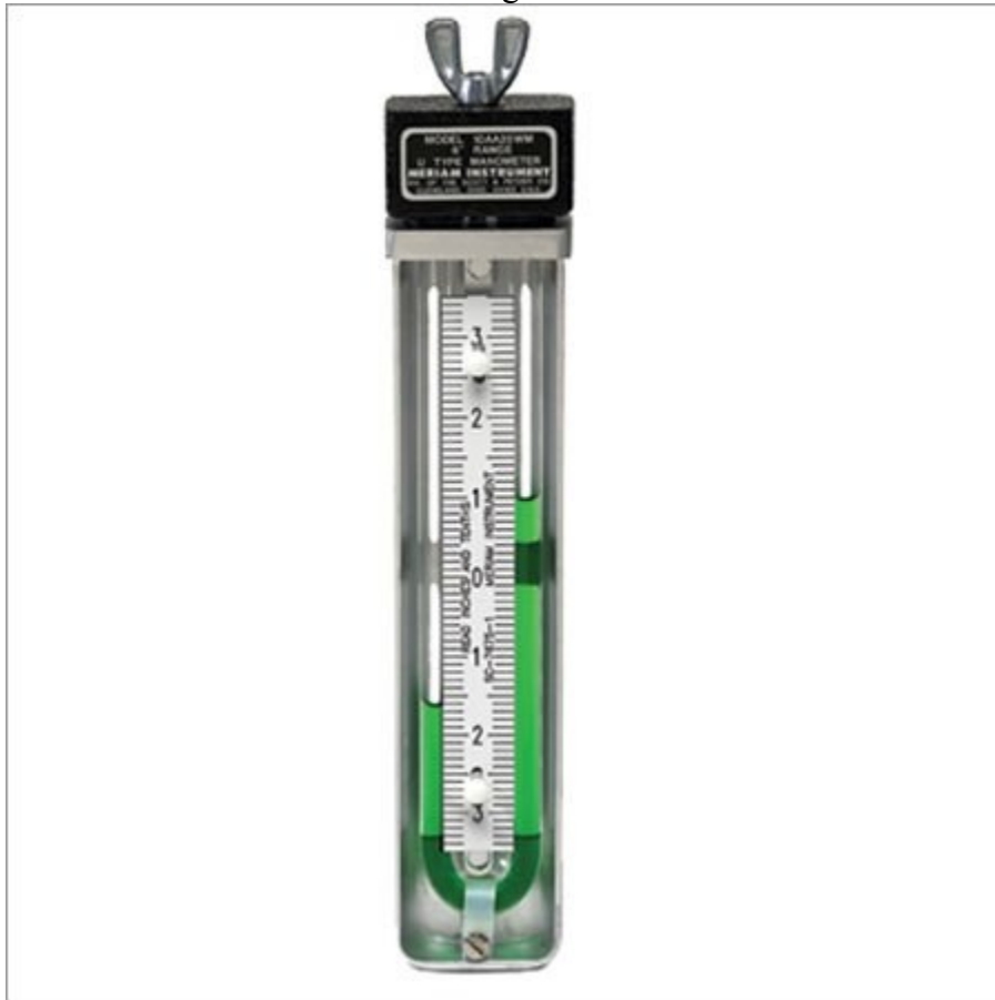
U-Tube Manometer with height markings Courtesy of Sharpinstruments
