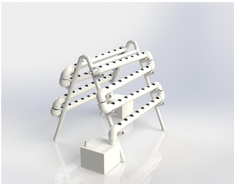
Figure 5: 3D Render of our Hydroponics System from Solidworks.
