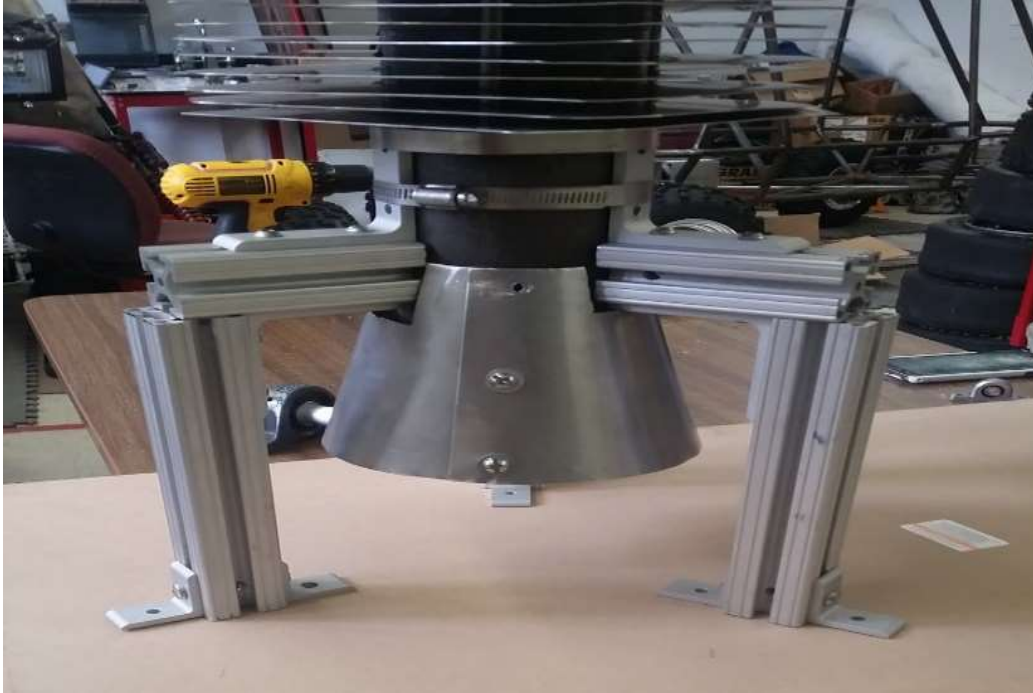
Figure 74- View of Shroud and Cylinder Supports
