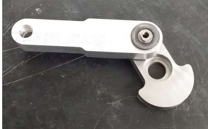
Figure 62-Power Piston Connecting Rod attached to End Crank
