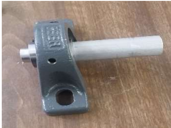
Figure 59- Turned stock in Pillow Block Bearing
