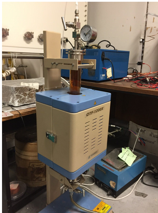
Fig. 4. Tube furnace in use. The brown gas is nitrogen dioxide, indicating that the nitrate has decomposed.
