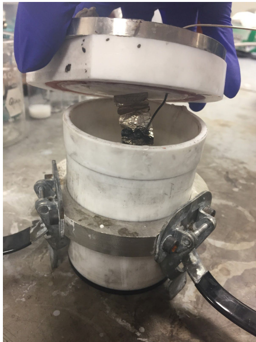
Fig. 3. Image of an open electrolytic cell, showing the platinum foil
