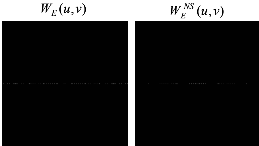
Figure 6.26 2-D Electronic NPS with the structure noise [ W_E(u, v) ] and without the structured-noise [ W_E^{NS}(u, v) ].
