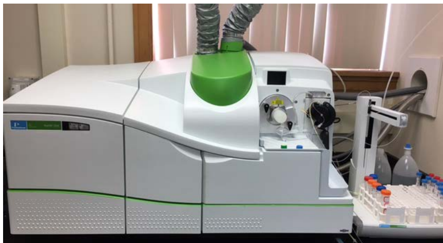
Figure B7-1. ICP-MS instrument for the analysis of metallic elements in wastewater and digested sorbents.
