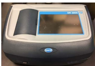
Figure B4-1. UV-vis spectrometer used for the analysis of total ammonia and total phosphors.
