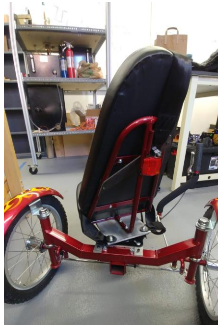
Figure 35: Rear view of seat frame with swivel mechanism.
