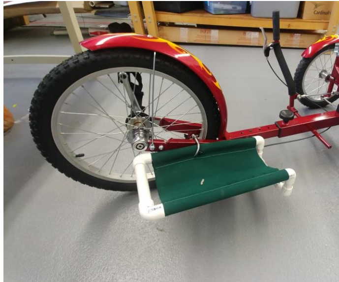
Figure 39: The sling sub assembly attached to the OEM frame.
