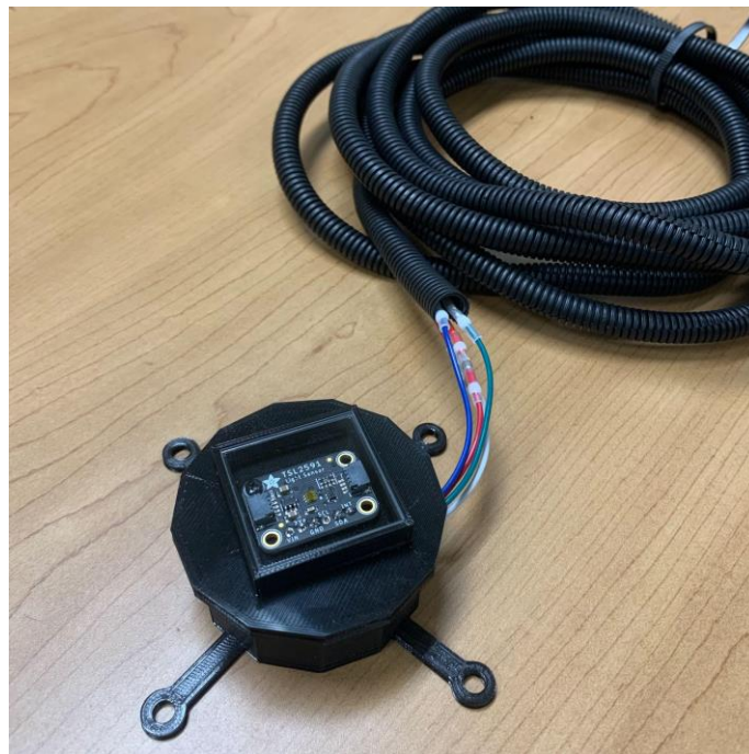
Figure 3. Light sensor in 3D printed enclosure connected to wires with ribbed sheathing.
