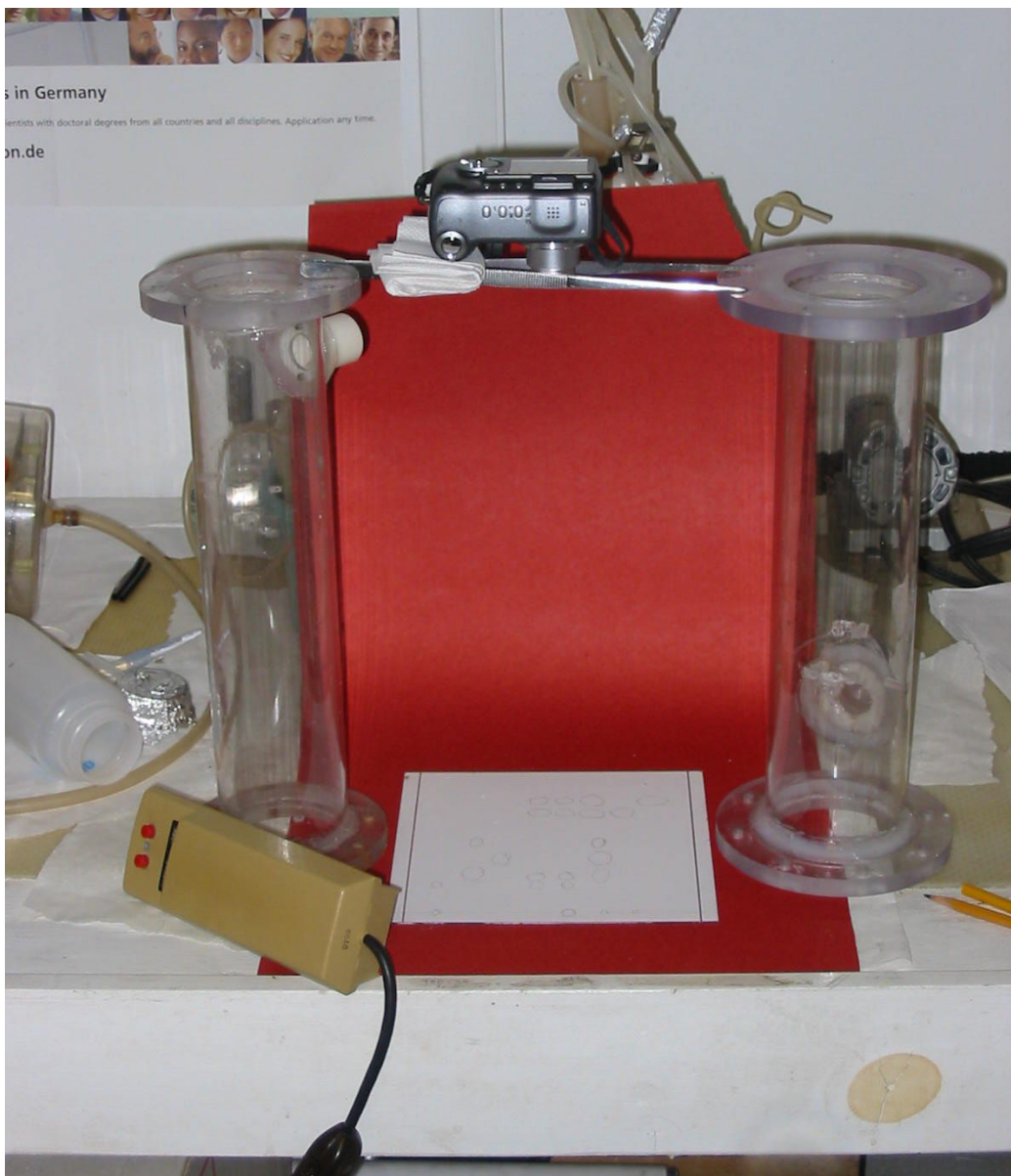
Figure 11: Side view of camera set up used to take long exposure TLC plate pictures under UV light
