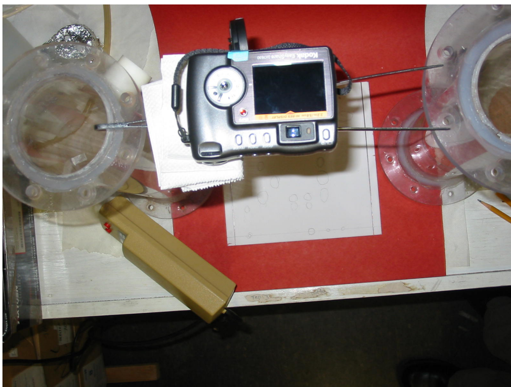
Figure 10: Top view of camera set up used to take long exposure TLC plate pictures under UV light
