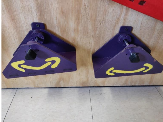
Figure 38: Final teeter totters fastened with circular mounting pieces and metal rods.
