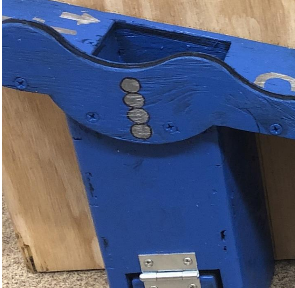
Figure 24: Counting ramp with visual of how plastic balls inside ball tower is supposed to be stacked.
