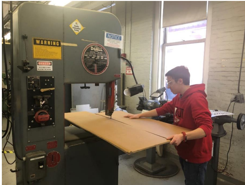
Figure 29: Spencer using the bandsaw in Washburn Shops to break down large sections of cardboard to fit into the laser cutter.
