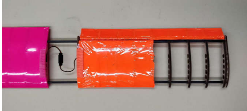
Figure 45. Structure of wing with MonoKote removed
