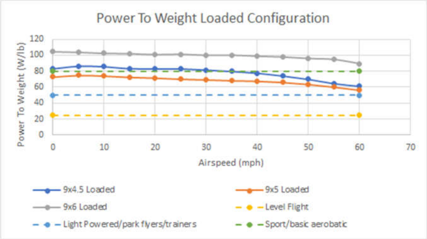
Figure 66. Power to Weight Loaded
