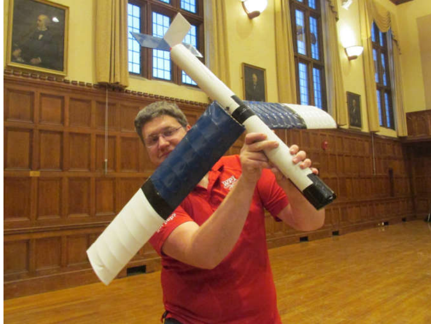
Figure 61. Glide prototype after repeated glide tests. Note: wing spars cracked, and nose cone was replaced with duct tape after it shattered
