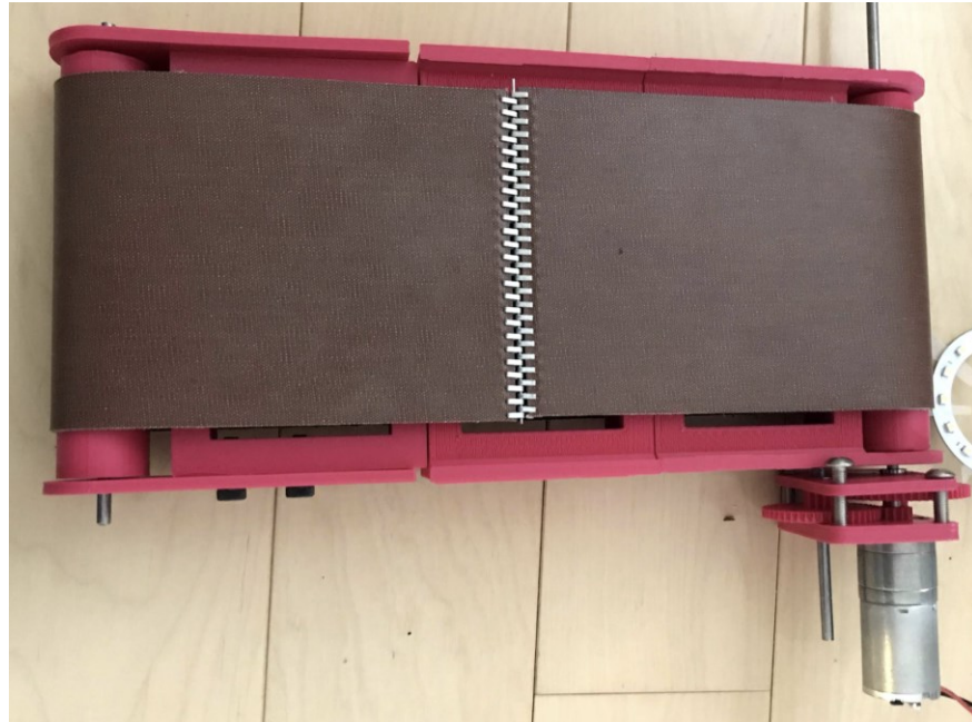
Figure 9: Serializer, Belt Construction Prototype
