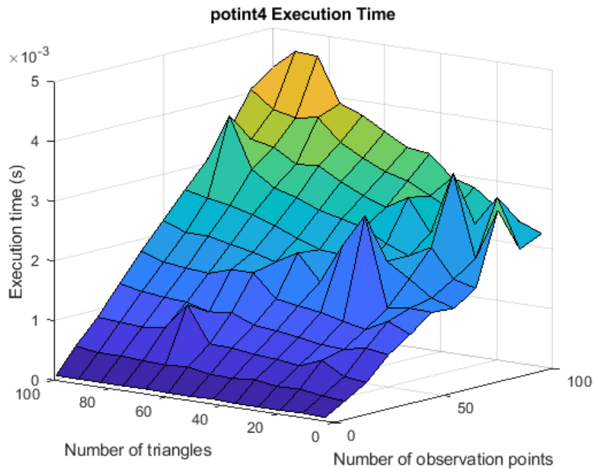
Fig. 13. Execution time for the triangle-vectorized solid angle approach ( potint4 ) as a function of number of observation points and number of triangles, bounded to 100 observation points and 100 triangles to present a more typical use case. Note that the vertical scale is one-sixth that of Fig. 12.
