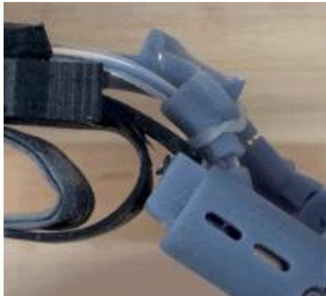
Figure 27: Flexing element under passive deformation.
