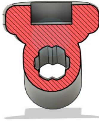
Figure 12: Section view of bowden tube link (5).
