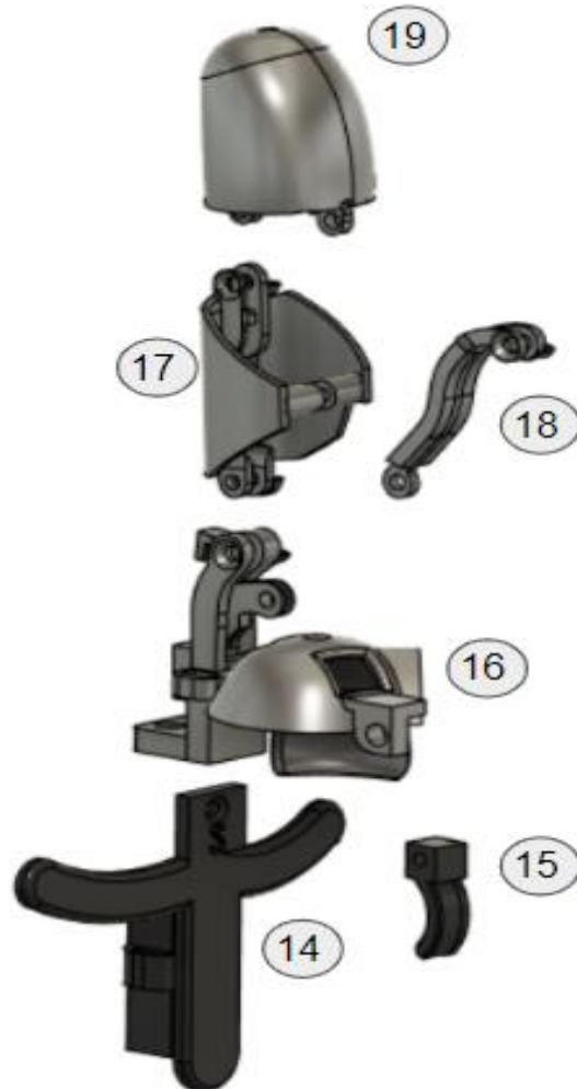
Figure 5: CAD rendering of thumb with individual components labeled.
