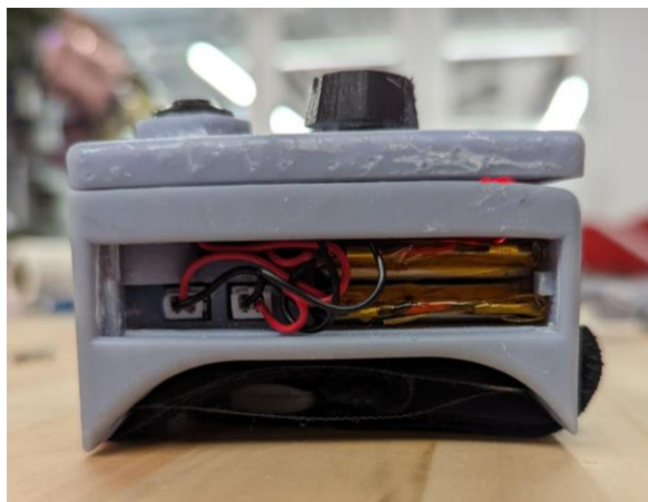
Figure 22: Wrist module with battery cover open and batteries plugged in.
