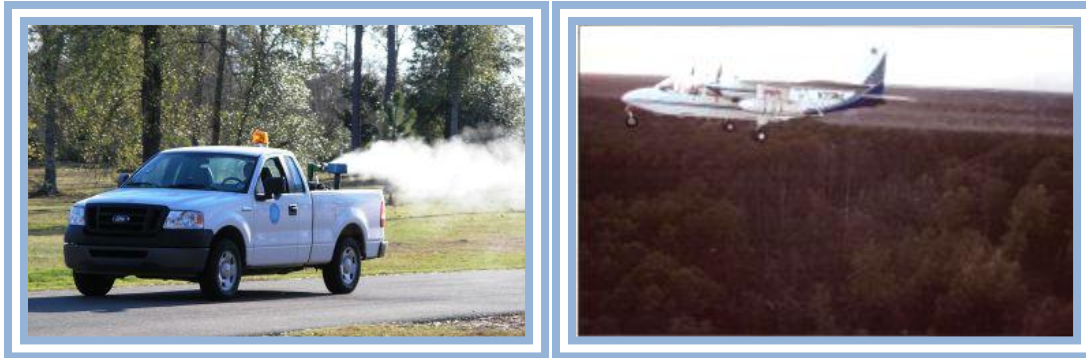
Figure 4: Photographs of Ground-Based Ultra Low Volume Spray (left) and Aerial ULV Spray. Figure from St. Tammany Parish Mosquito Abatement District (n.d.)
