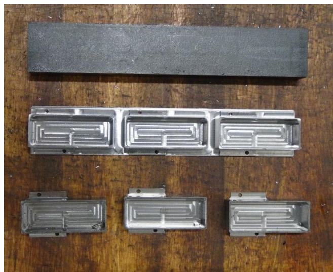
Figure 7: Raw Stock to Finished Part
