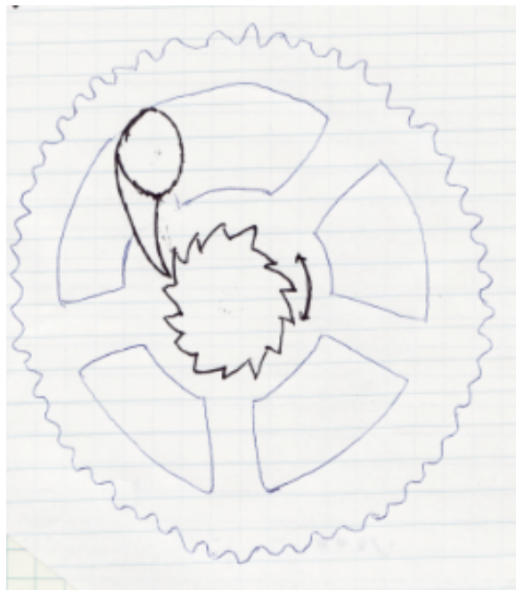
Figure 33 - Ratchet idea. This design would have ratchet connected to a gear.
