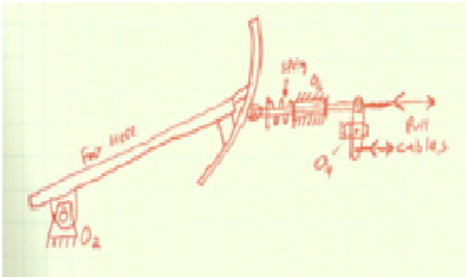
Figure 20 – Foot-controlled, cam actuated cable system. This design uses a foot pedal to control a cam that actuates the cables for a cable system.
