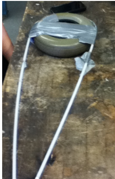
Figure 76 - Set up for test to determine how much force is required to push pseudo-fluid balls around a bend with a 3.75" Radius.
