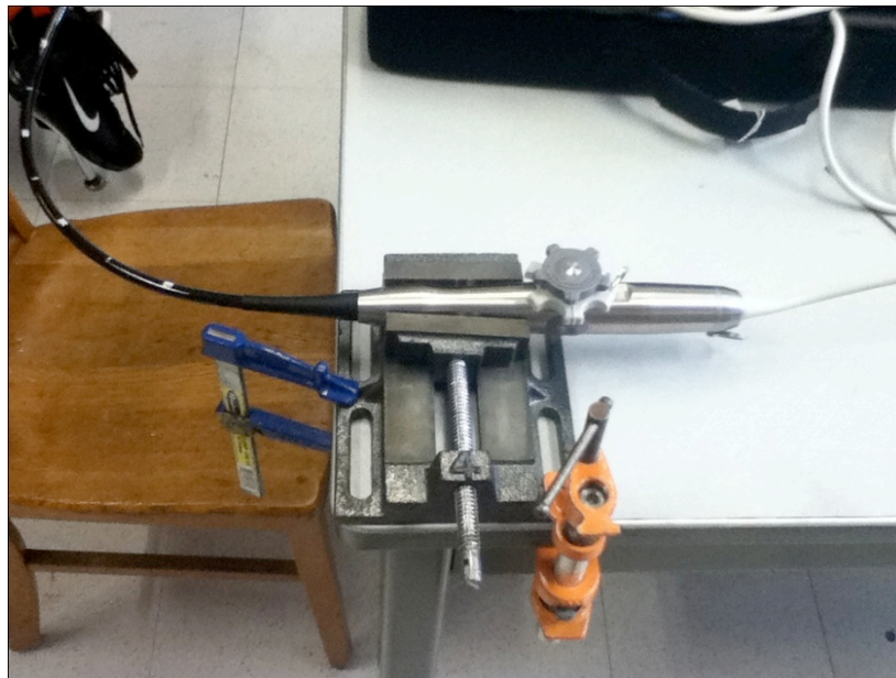
Figure 72 - Set up for the test to determine how much torque was required to rotate the knobs of the TEE.
