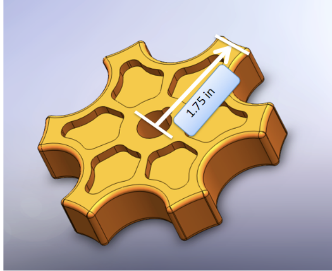
Figure 66 - Knobs of the pseudo-fluid control extension system, showing the radii of the two knobs from where they were pulled in the determination of how much torque was required to rotate the knobs.
