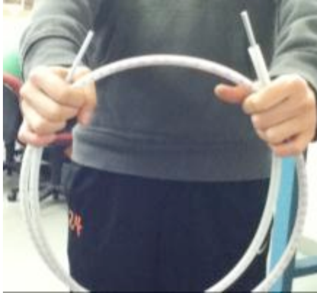
Figure 56 - Pseudo-fluid ball system. The system consists of a plastic tube filled with small ball bearings that can be pushed back and forth by pistons. This system is advantageous because provides advantages of cable and hydraulic systems and does not include disadvantages such as leaking (hydraulic) and stretch (cables).
