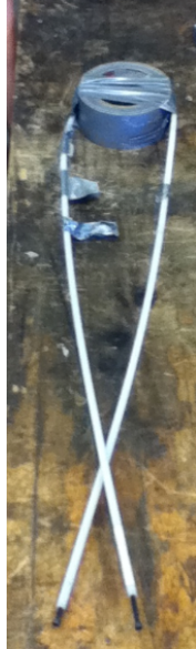
Figure 77 - Set up for test to determine how much force is required to push pseudo-fluid balls around a bend with a 2.34375" radius.
