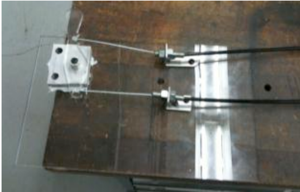
Figure 54 - Rocker Handle- User Interface of the Rocker Handle System zeroth order prototype, showing handle, cables, and tensioning system.
