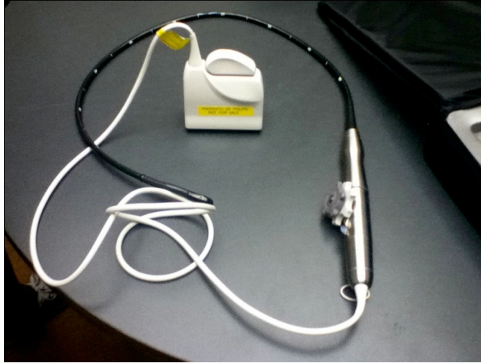
Figure 9 - Transesophageal echocardiogram probe. The TEE consists of a black probe that is inserted into a patients esophagus, a ultrasound transducer located at the distal end of the probe, a silver handle with two rotatable knobs that control the motion of the probe, and an electrical connection that connects to a computer.
