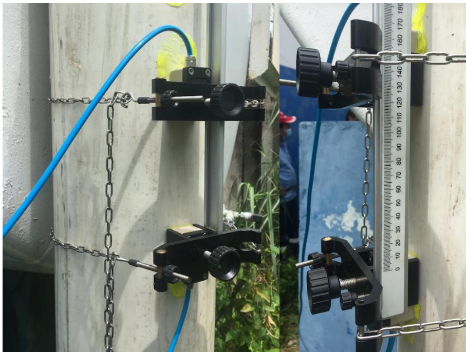
Figures 3.2-3. The setup for the flow meter measurements. With the help of IDAAN's engineers and workers, we operated these devices to measure flow rate, in gallons per minute.
