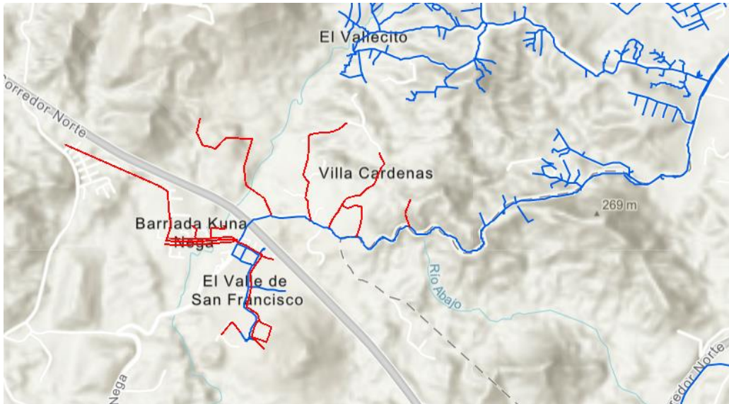
Figure ES.1. ArcGIS model of existing hydraulic pipelines. Blue lines reflect pipes that existed in the model already, and red lines reflect pipes that we added.
