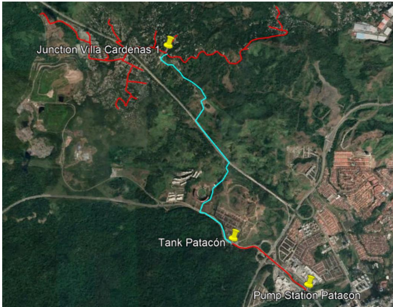
Figure 3.17. How the Patacón Pump Station (Pump Station Patacón) could connect to the existing system. The red lines represent existing pipelines, the blue line is the proposal. This route takes into account IDAAN's design plans to intercept the system at the Villa Cardenas 1 Junction, mitigates extraneous altitude changes, and follows existing roads as closely as possible.
