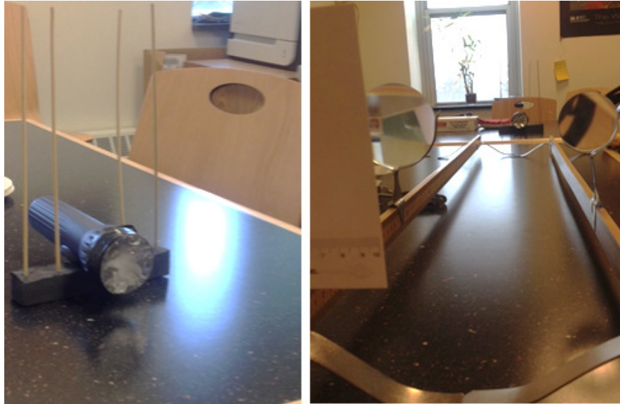
Figure 6: Flashlight set up 5-8 away from the work station including two adjacent meter sticks, two lenses and a screen.
