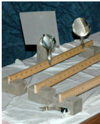
Figure 10: Move the screen to the side so that at least some of the light is hitting the mirror and an image form.
