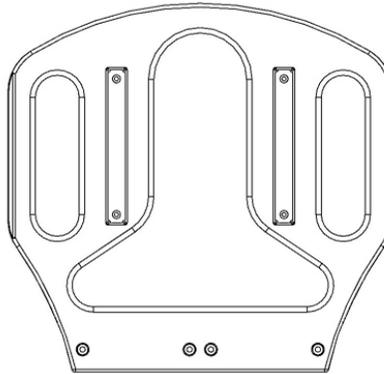
**Figure 4** – Bottom side view of the bottom half of the IBC housing.
