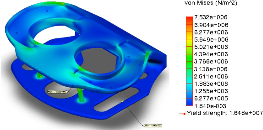
**Figure 6.2** - Finite element stress analysis of the housing during a side loaded patient scenario.
