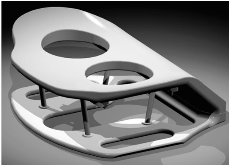
**Figure 8.1** - Final design of the InsightMRI breast coil housing concept.
