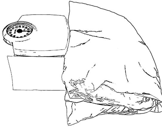
**Figure 4.2** - The setup used to determine chest weight loading on the breast coil.
