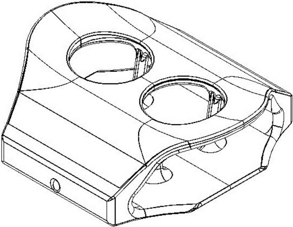
**Figure 5.3-** A symmetrical concept, allowing for feet- *or* head-first patient entry.
