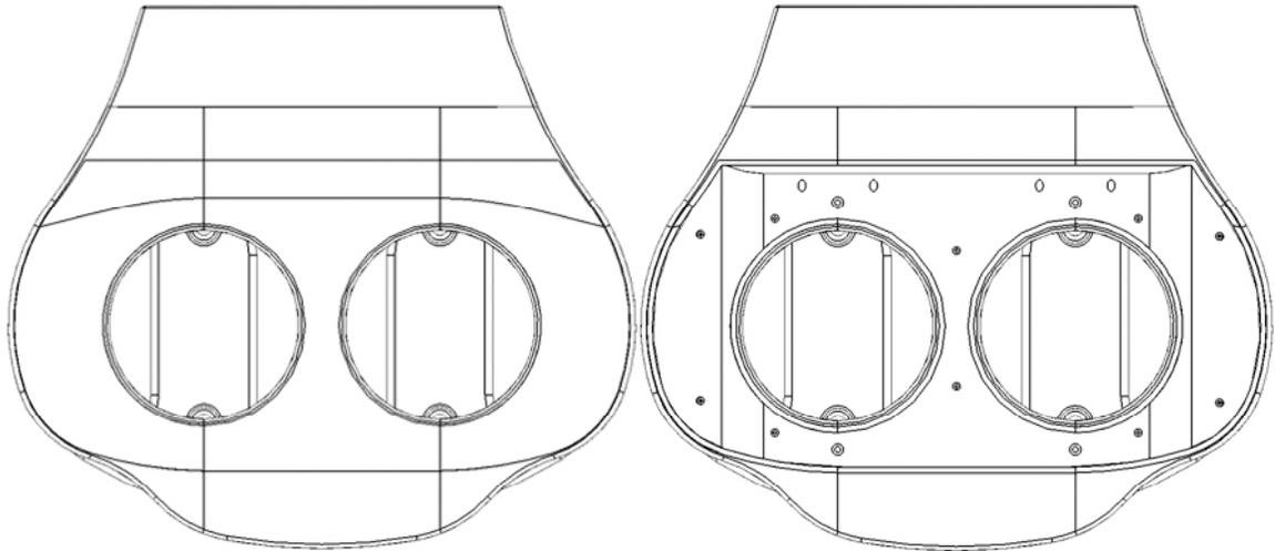
**Figure 5.6** - A top-down view of the top half of the housing showing the patient surface (left) and the internal electronics cavity (right).
