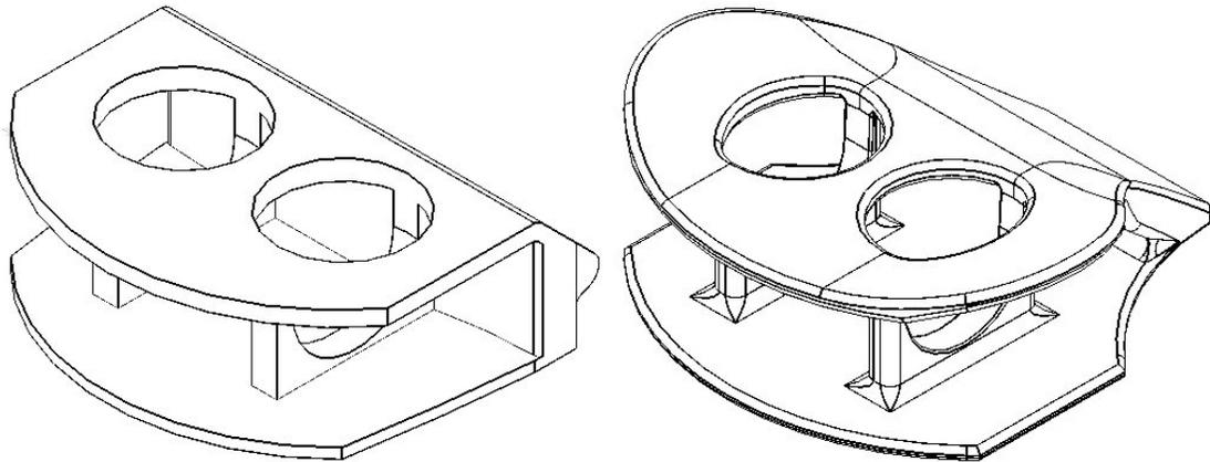
**Figure 5.2-** The second conceptual design with (left) a simplified model and (right) an ergonomic revision of the simplified model.
