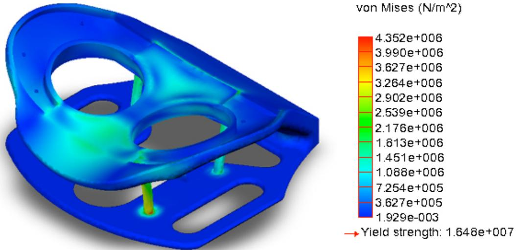
**Figure 6.1** - Finite element stress analysis of the housing during a top loaded patient scenario<sup>1</sup>.
