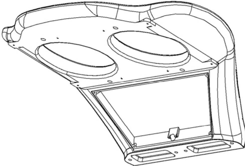
**Figure 5.7** - A bottom side view of the top half of the housing.
