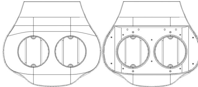
Figure 2 – Top surface of the top half of the housing, with the patient surface (left) and the electronics cavity (right).
