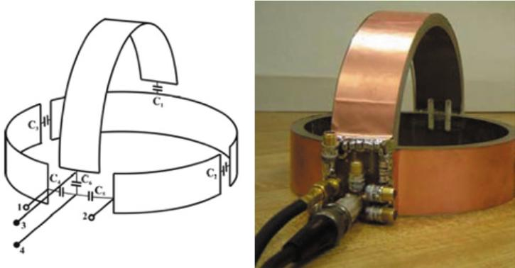
**Figure 2.8**– Dual-channel array coil concept (left) and model (right) (Obi, 2005).
