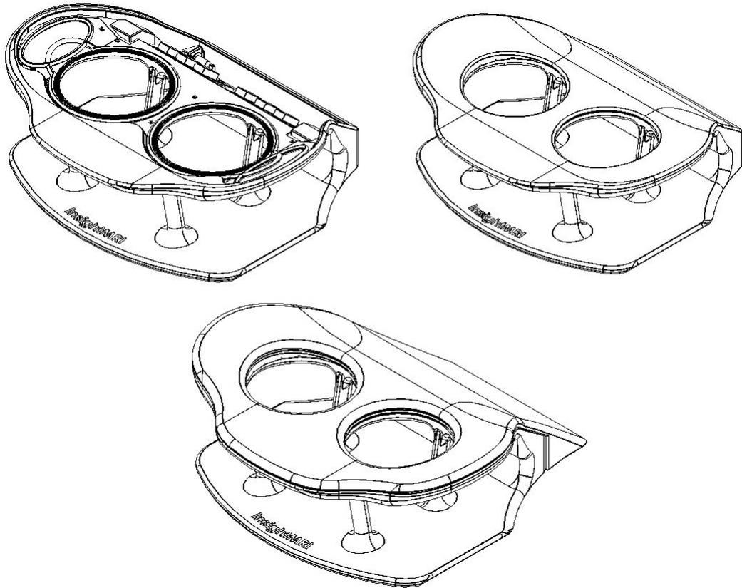
**Figure 5.4-** The last concept prior to a final detailed design, showing (top left) the device's internal cavity and electronics, (top right) the device with the top cover and (bottom) the device with ergonomic foam support.
