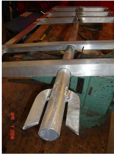
Figure 29: Aluminum Welds on Wings
