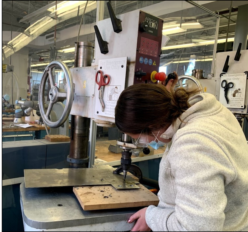
Figure 36: Using the drill press to cut holes in the outer casing
