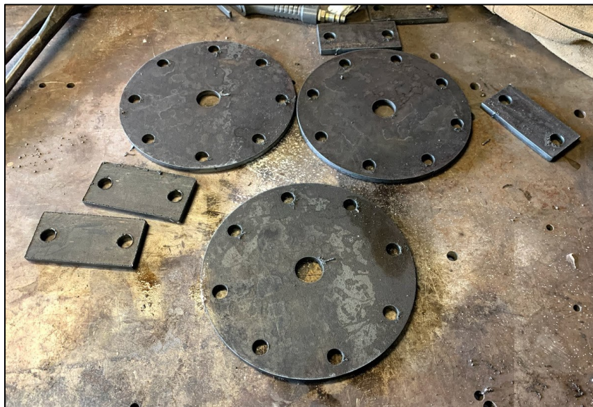
Figure 33: Hammers and rotor discs plasma cut out of the 1/4" thick steel plate
