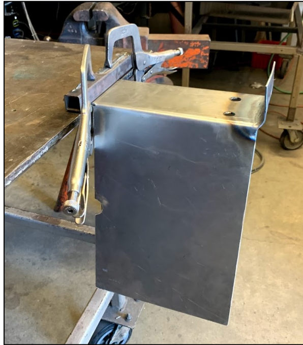
Figure 39: Outer casing clamped to the table, ready to bend the flanges
