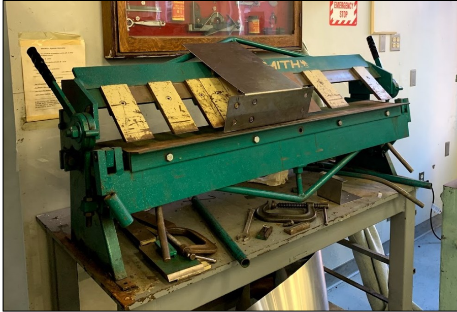
Figure 37: Sheet metal brake used in Washburn Shops
