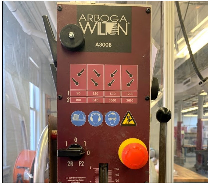
Figure 35: Front face of the drill press, showing the available feed rates and their settings
