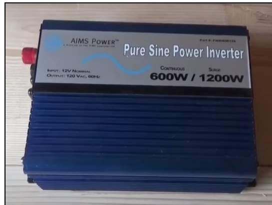
Figure 56: Pure Sine Power Inverter (Reid, 2017)
