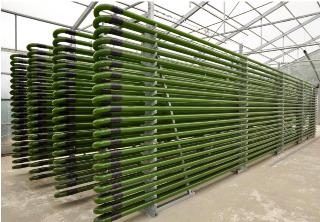
Figure 10: This is a tubular photobioreactor built for IGV Biotech in Germany.
