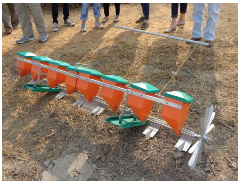
Figure 15: Rice Sowing Machine
