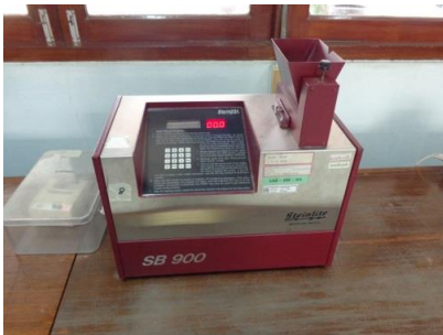
Figure 11: Moisture Content Machine
