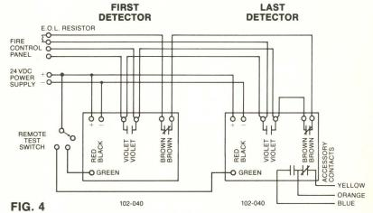
TYPICAL CONNECTION FOR A LOW VOLTAGE MODEL 40 DETECTOR WHEN USED IN A FOUR-WIRE DETECTION CIRCUIT WITH RETURN WIRING IN THE SAME CIRCUIT.
