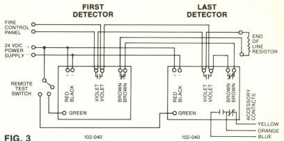
TYPICAL CONNECTION FOR A LOW VOLTAGE MODEL 40 DETECTOR WHEN USED IN A TWO-WIRE DETECTION LOOP.
