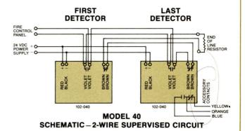
\*NOTE: Wiring for Model 104-040 identical to above except power connections are either 120 volts AC to blackwhite leads or 24 volts AC to black/yellow-white leads.
