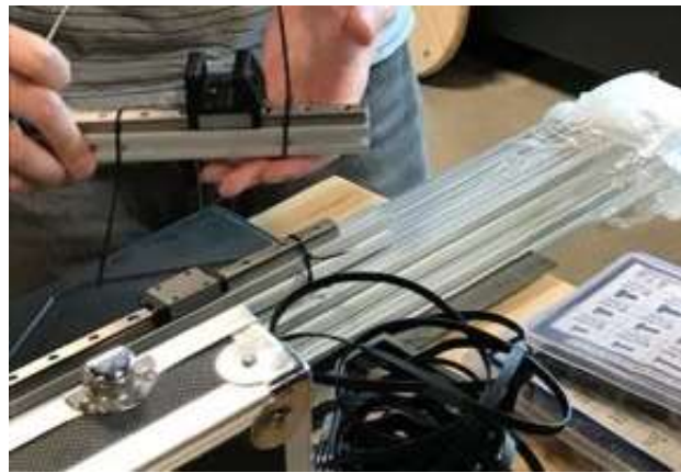
Figure 20. Aluminum extrusion and linear bearing
