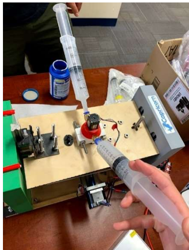
Figure 4. Manually entering silicone parts A and B using syringes.
