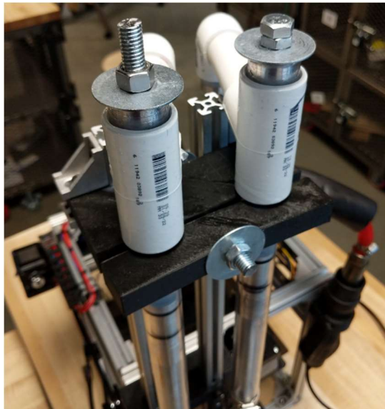
Figure 14. The bleed port, which was added the final iteration, is pictured. Specifically, the bleed port plug bolts can be seen at the top of the apparatus. These bolts can be easily removed to reveal a port through which silicone can be added to the system and air can be removed.
