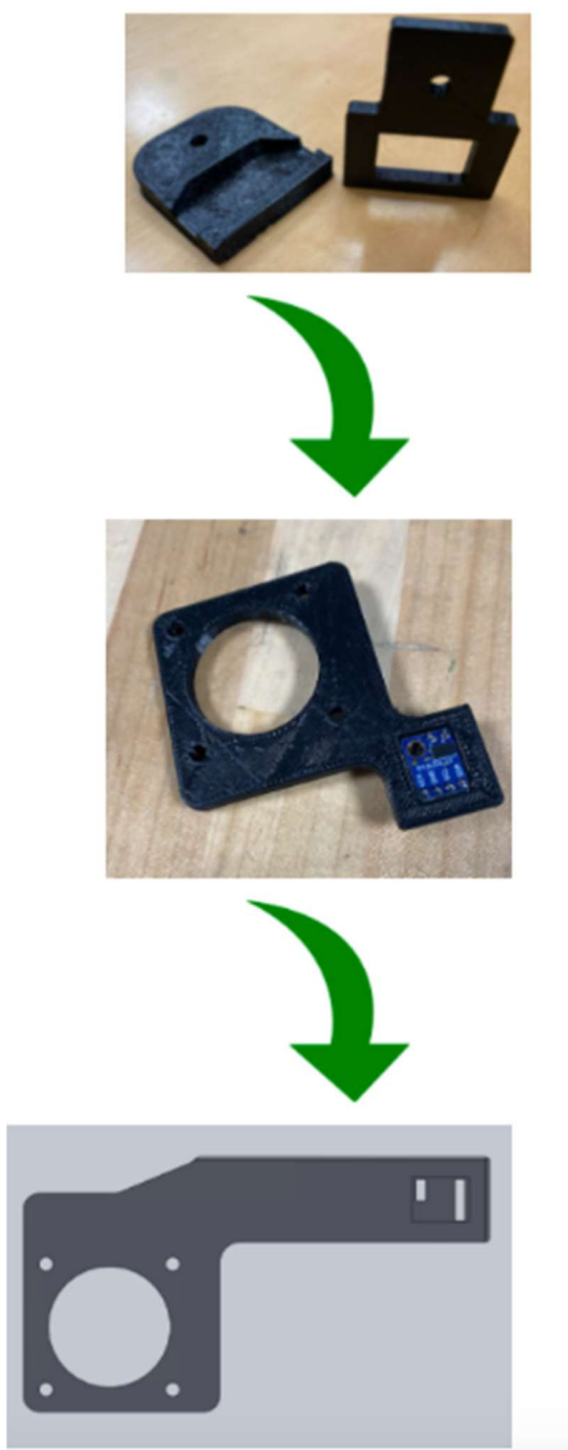
Figure 38. Evolution of the v153loz TOF sensor casing
