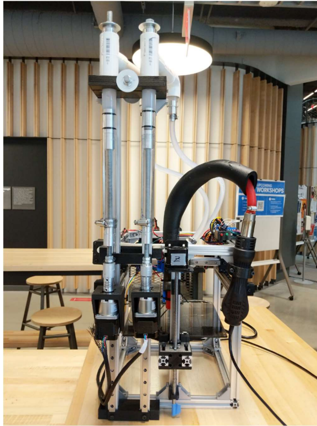
Properly installed extruder (1)
