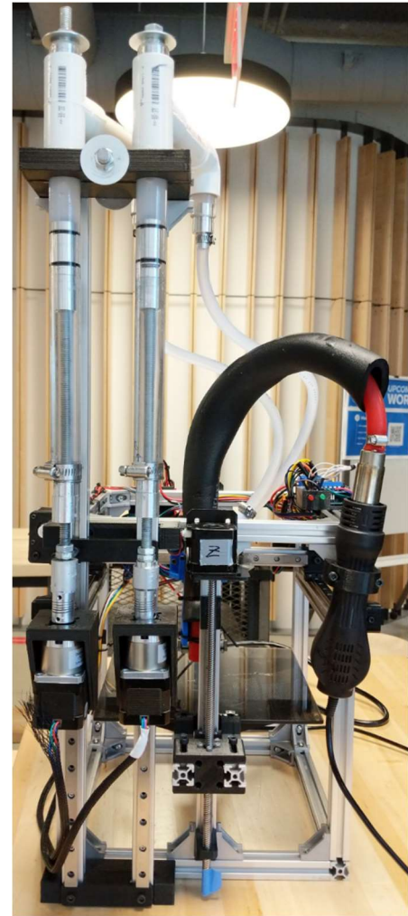
Figure 15. Pictured is the final version of the extruder assembly, mounted to the printer. Near the top of the photo are the bleed ports which were added for the final iteration.
