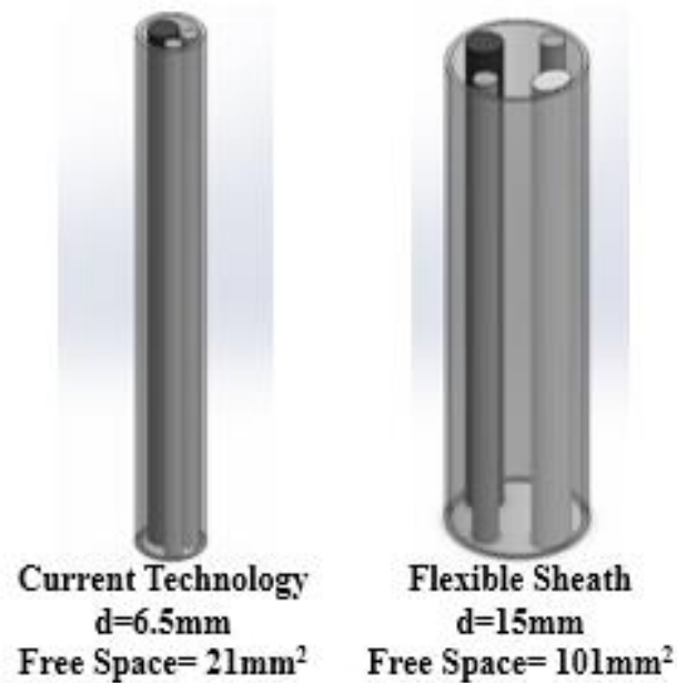
Figure 29: 5x increase of free working space with new design and use of larger surgical tools
