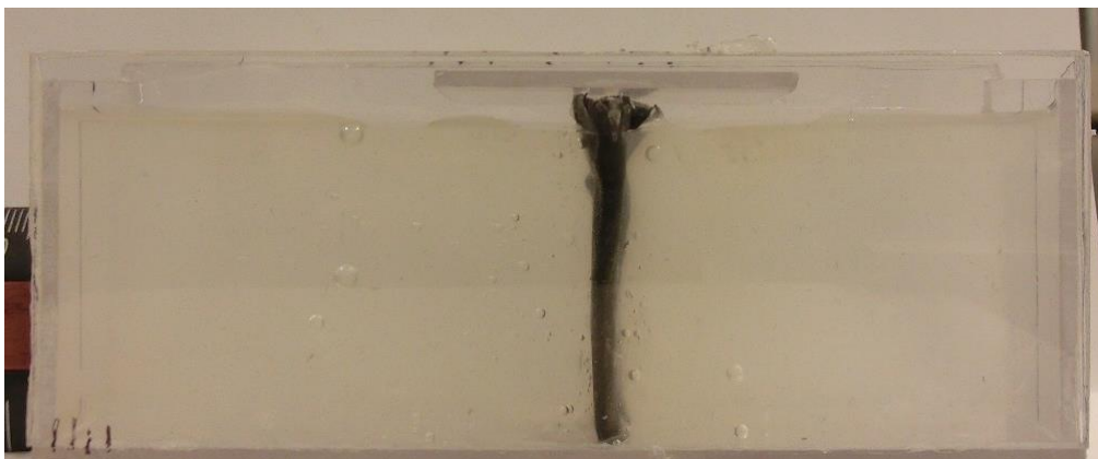
Figure 30: Collapsed PTFE Sheath in Gel
