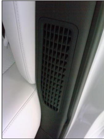
Figure 28: Vents for Battery Pack in Rear Seats of Lexus Model HEV (Northborough)
