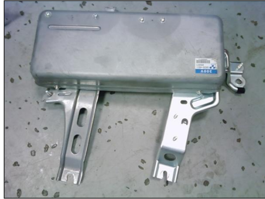
Figure 7: DC-DC Converter (Northborough)
