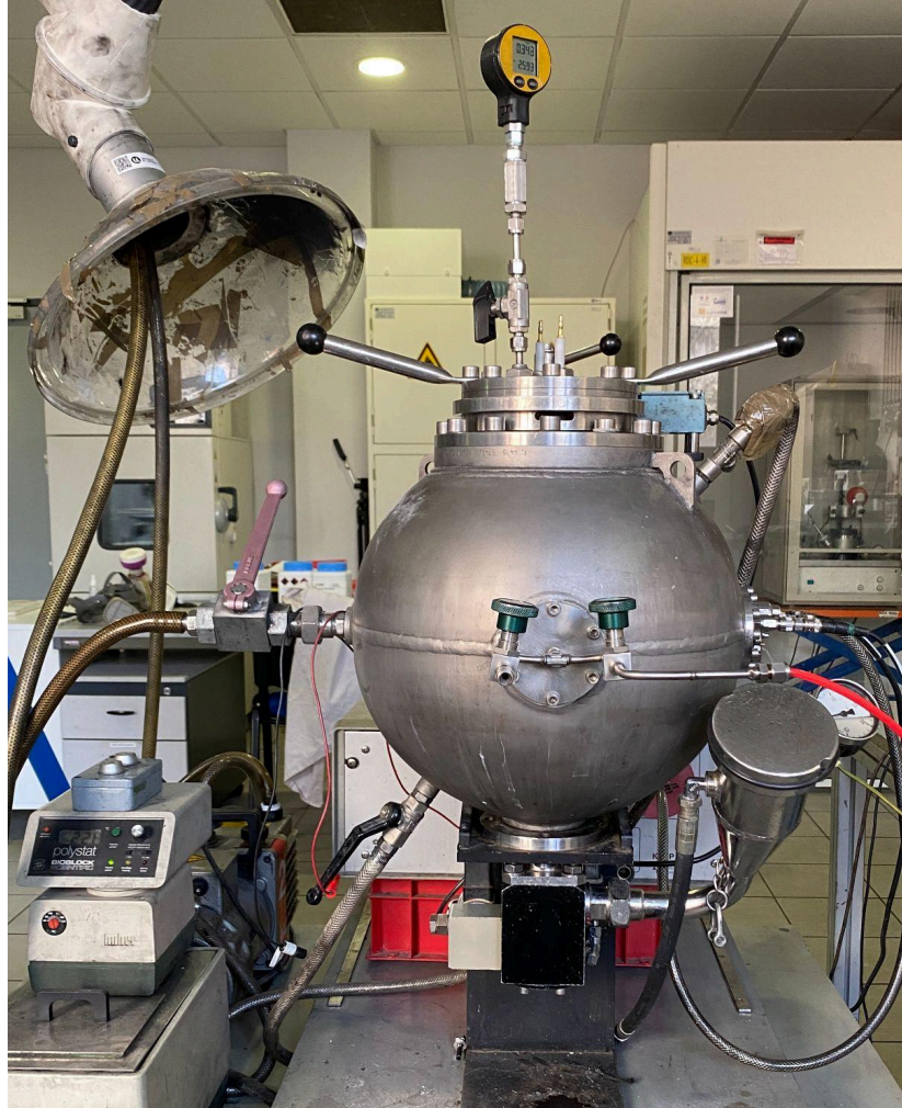
Figure 1.2: Picture of the 20-L sphere apparatus used
