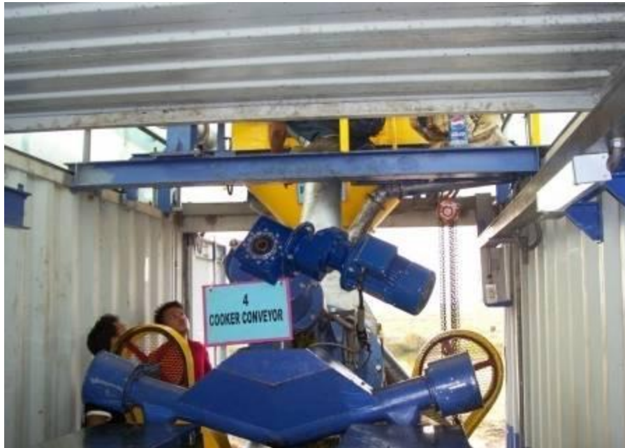
Figure 25: Demesocarper to remove nut from fruit (yellow machine in back) and cooker conveyer to warm fruit.
