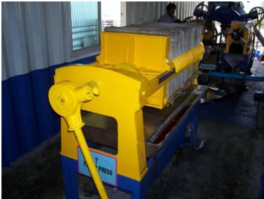
Figure 28: Filter press to filter fine material.
