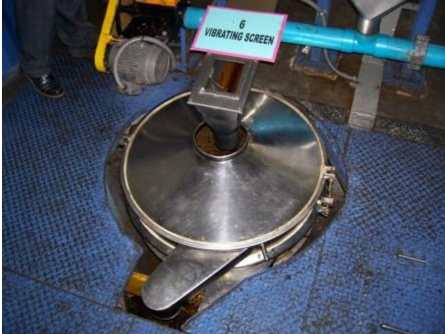
Figure 27: Vibrating screen to filter coarse material.
