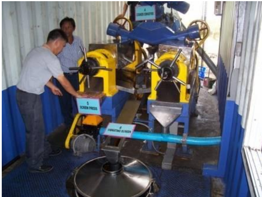
Figure 26: Cooker conveyer to warm fruit, screw press to extract oil, and vibrating screen to filter coarse material.
